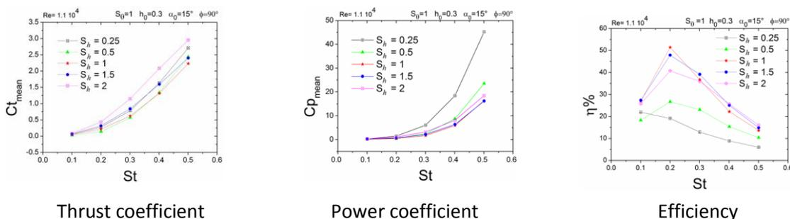
Figure 4. Effect of non-sinusoidal heaving on the propulsive performances
