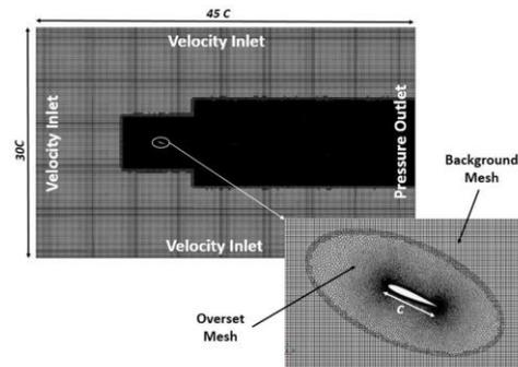
Figure 2. Computational domain with overset mesh
