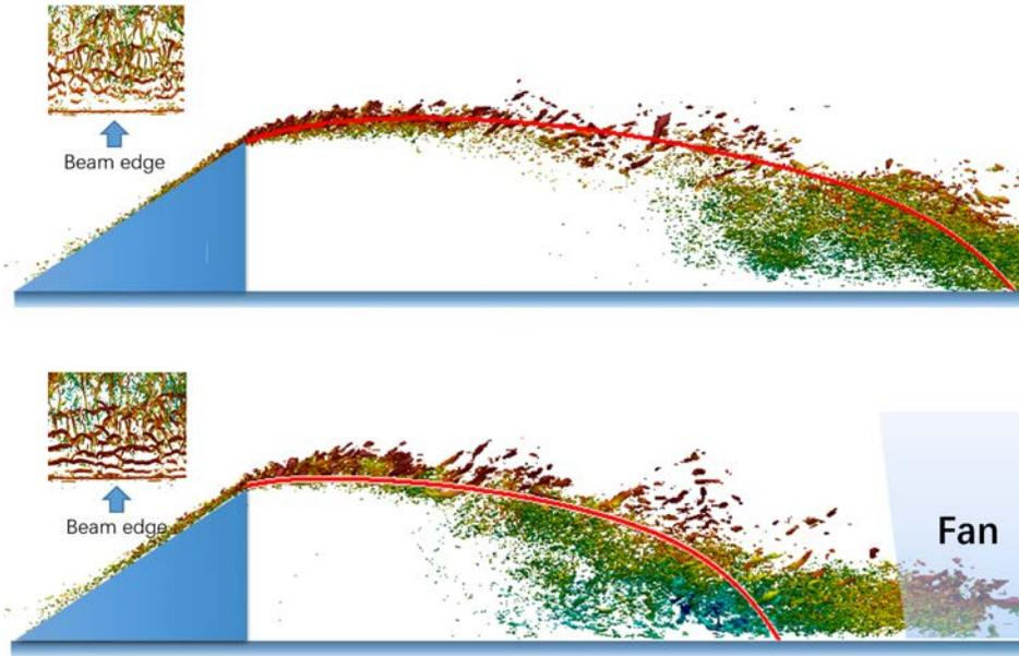
**Figure 4.** Lateral view of instantaneous flow for the case without fan and with fan
