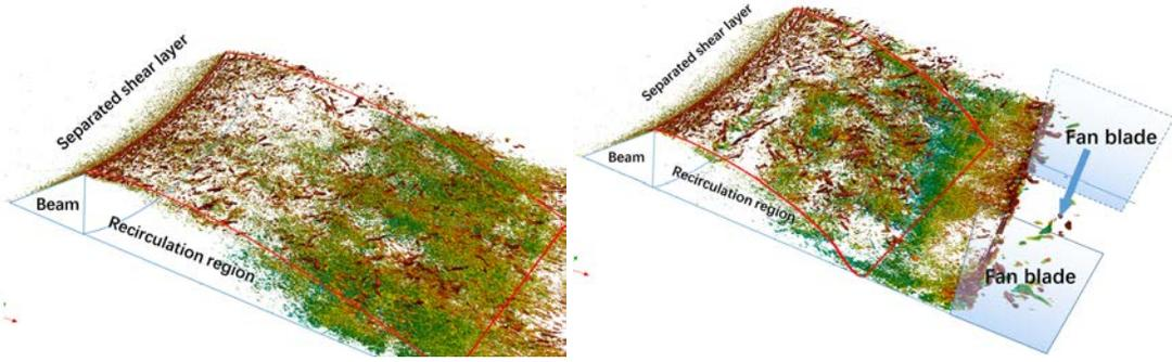
**Figure 3.** Instantaneous flow for the case without fan and with fan
