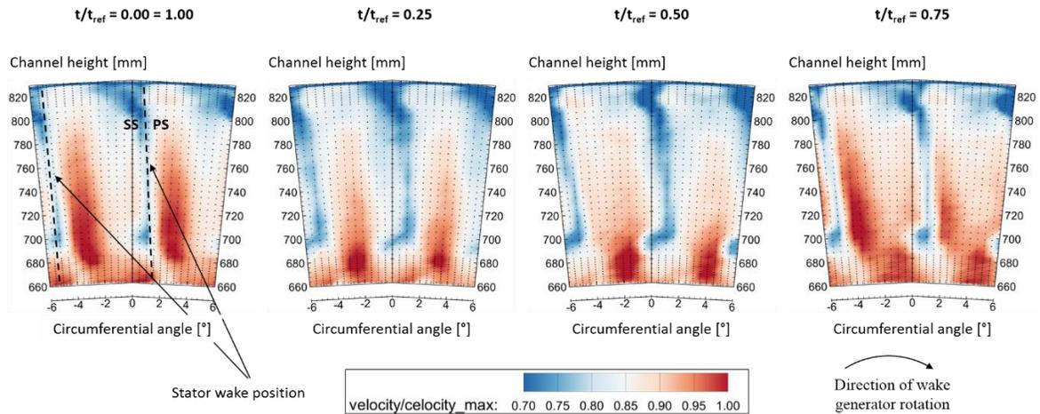
**Fig 2. Time-resolved results in stator exit plane. Temporal evolution of non-dimensional velocity for one bar passing, divided into 4 time steps.**
