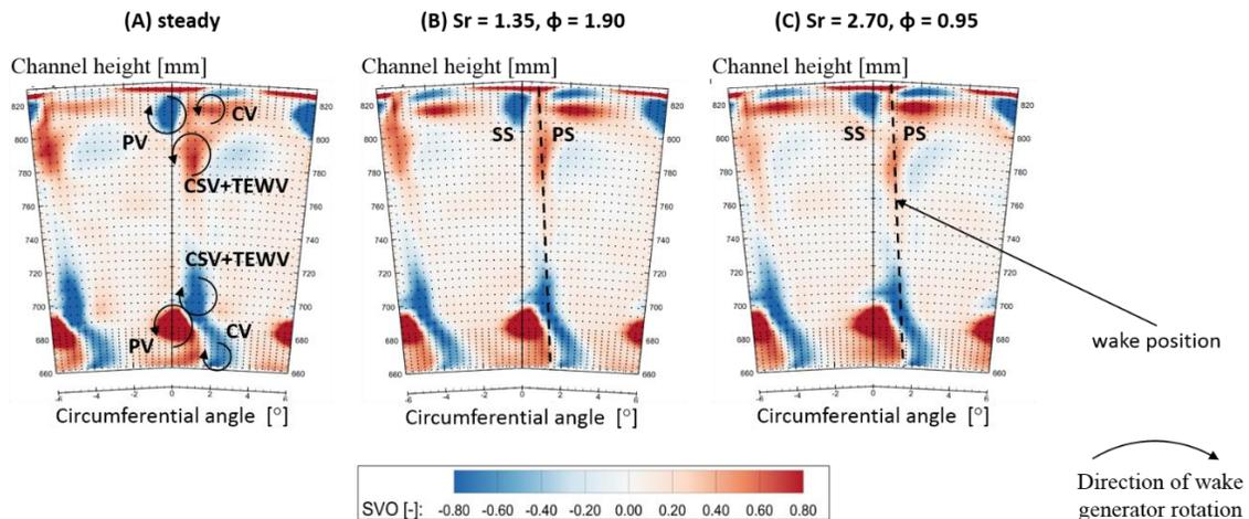
**Fig 3. Time-mean results in stator exit plane. Vorticity for undisturbed case (left, A) and for two cases disturbed by bar wakes (mid, B and right, C).**
