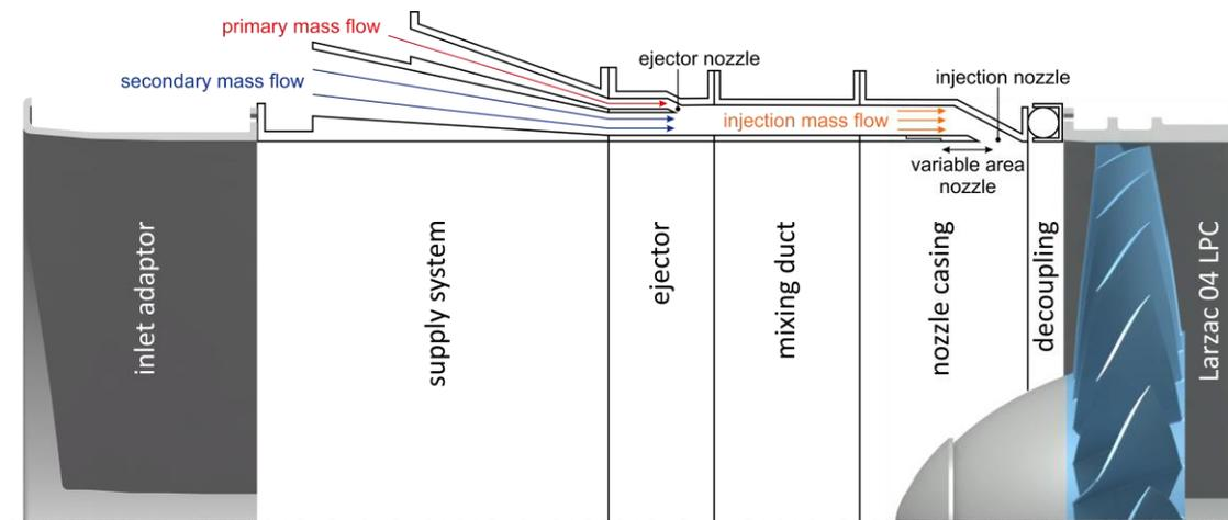
Figure 1. Schematic of the EIS
