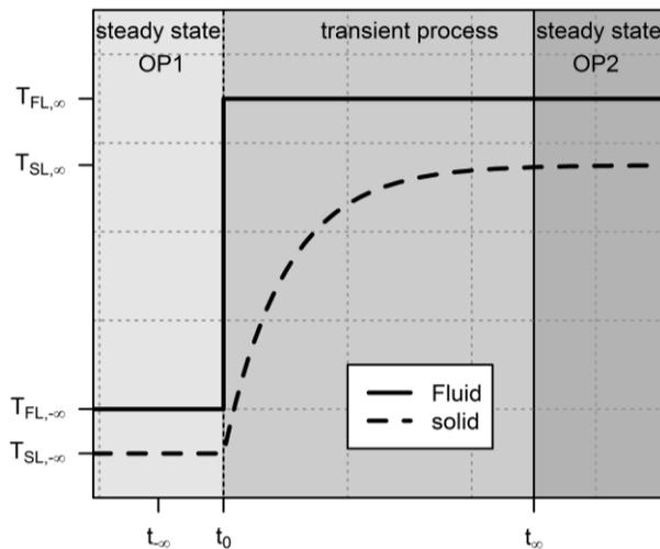
**Figure 1.** Qualitatively idealized behavior of fluid and solid temperatures in a thermal shock test [2]
