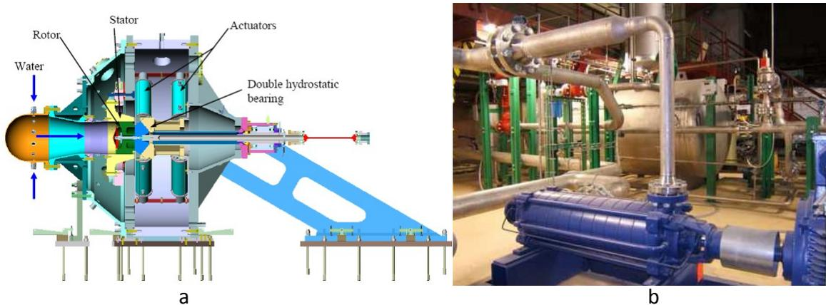
**Figure 1.** Cross sectional view of the test rig a) and view of the hydraulic loops b)
