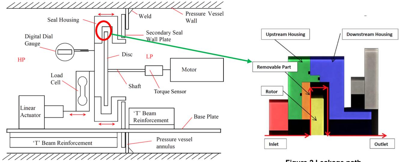
Figure 1 Non-Contacting Seals Rig Schematic.
