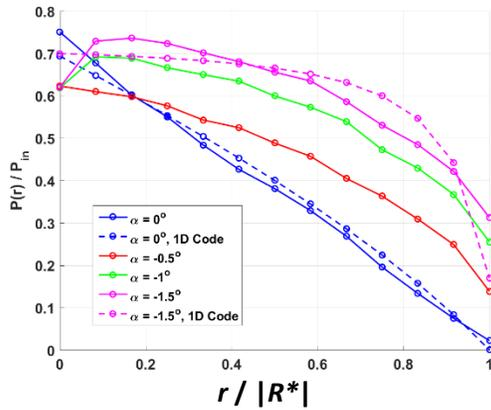
**Figure 3 Experiments, Converging coning, Radial pressure distribution,  $h_{\min}=100$ ,  $P_{\text{in}}=2.07$  barg.**
