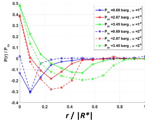
**Figure 4 Experiments, Diverging coning, Radial pressure distribution,  $h_{\min}=100\mu\text{m}$ ,  $\alpha = +1.0^\circ$  and  $\alpha = +2.0^\circ$ .**
