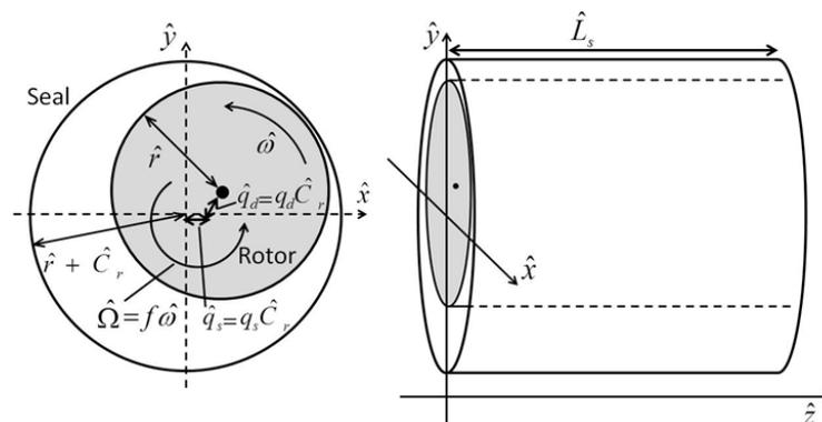
Figure 1. Annular Seal model and definition of parameters and variables
