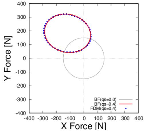
(a) Orbit of RD fluid force in xy plane
