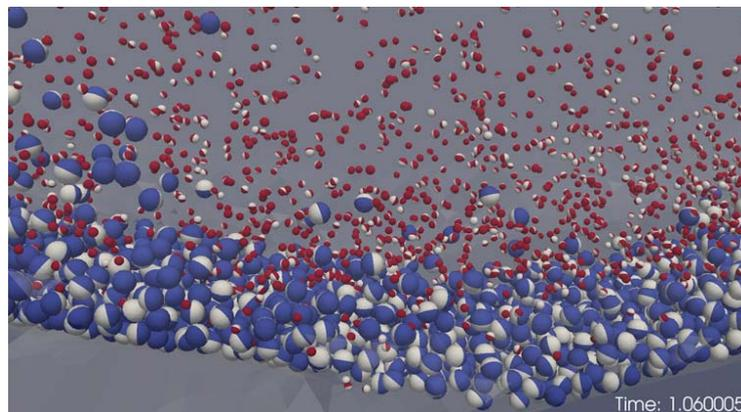
**Figure 1.** CFD-DPM simulation of a bidisperse rotating fluidized bed in a vortex chamber.
