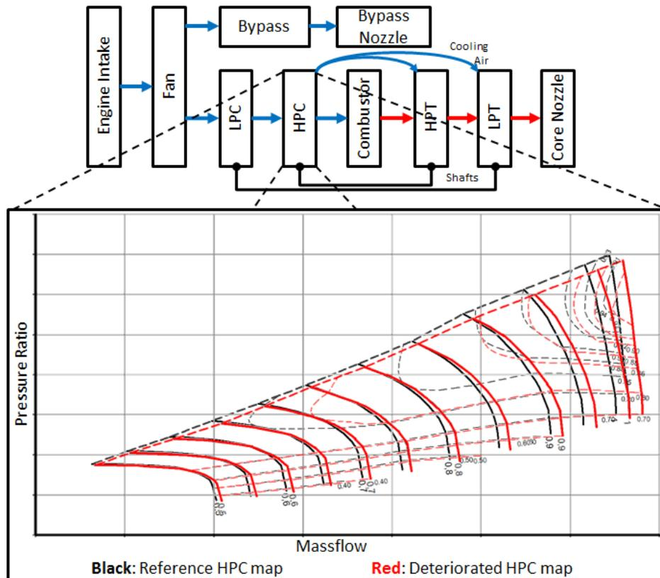
**Figure 1.** Scheme of a modular performance synthesis model with modified HPC maps
