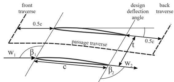
**Figure 2.** Definition of cascade and flow parameters
