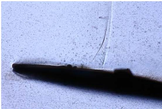
**Figure 1.** Shadographic image of the passage shock at high blade loading with dry but droplet-laden air.
