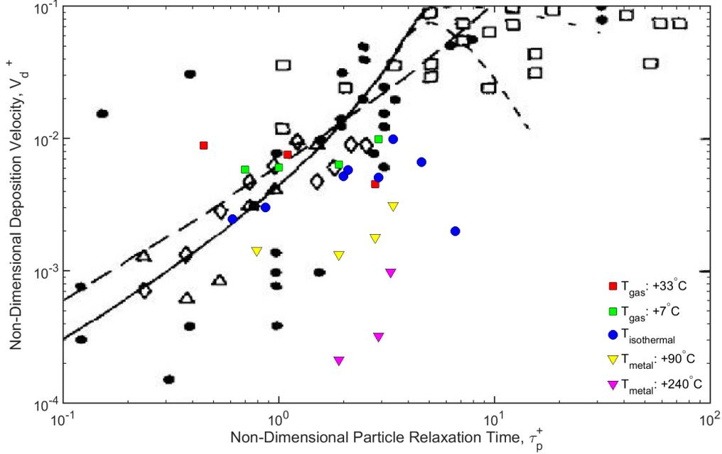
**Figure 1.** Experimental data for deposition of NaCl particles at engine-representative temperatures.  $T_{gas} = 390^\circ$ . Black shapes indicate experimental data of Kvasnak et al. [4].
