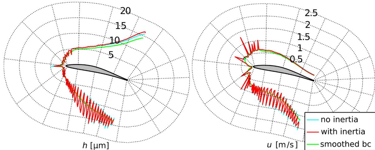
**Figure 1.** Wall film properties for different modelling approaches [2]
