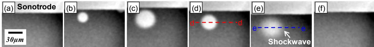
**Figure 1.** Six consecutive images, showing the oscillation and implosion of a bubble in a single wave period (an exposure time of 500 ns, and a time interval of 7.4  $\mu$ s between the consecutive images).
