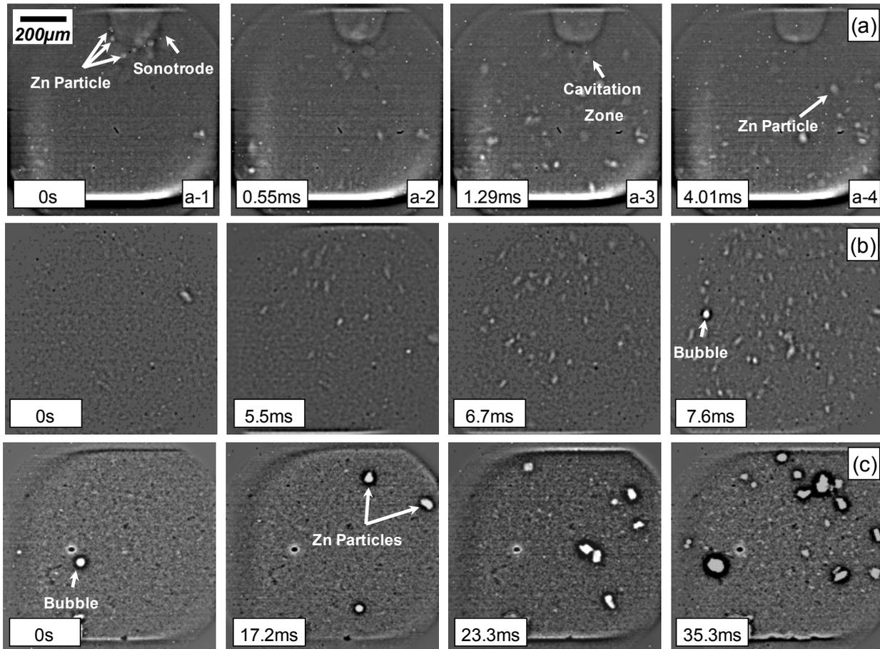
**Figure 2.** A series of images captured in liquid Bi-8 wt. %Zn alloy with an ultrasound power of 20 W at APS using 5413 fps. The images were taken at (a) 0.5 mm, (b) 2.5 mm, and (c) 4.5 mm respectively below the sonotrode tip.
