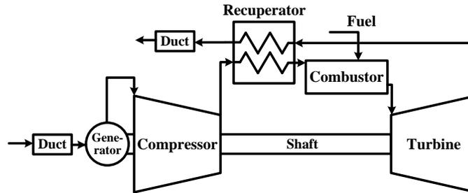
**Figure 1.** Schematic diagram of a micro gas turbine
