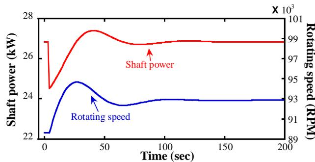
**Figure 2.** Dynamic simulation results according to a sudden 5% internal leakage from combustor inlet to turbine inlet
