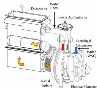
Figure 2. Perspective view showing arrangement of the main components of the microturbine [2]
