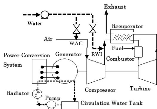
Figure 1. System diagram of the objective microturbine system [2]
