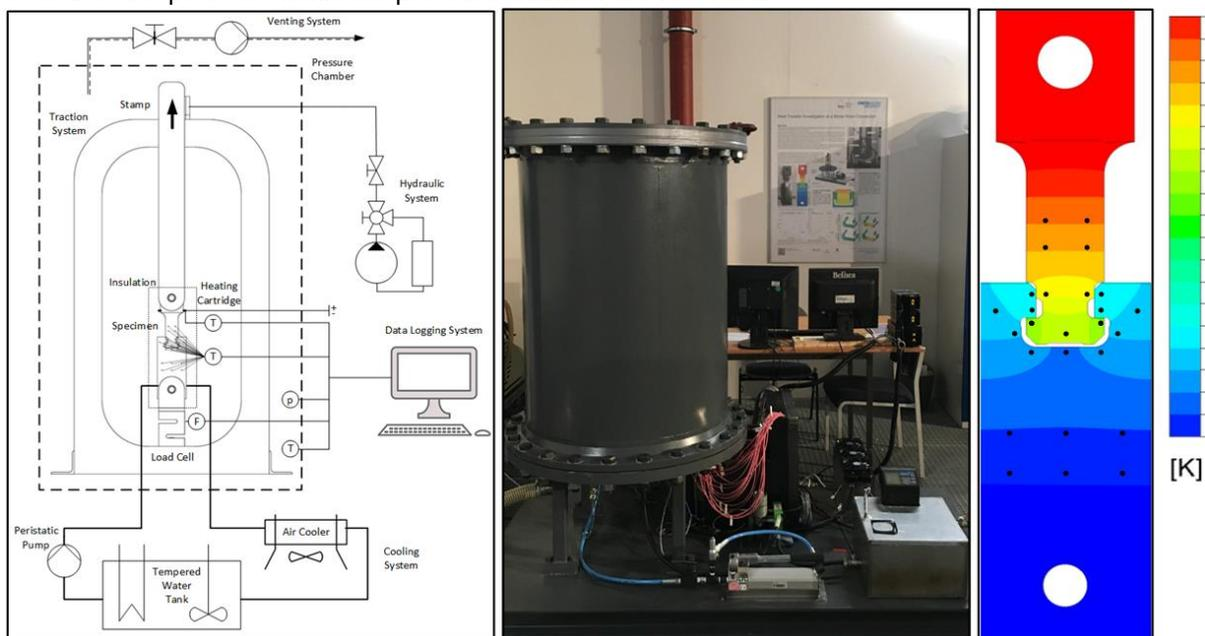
Figure 1: Schematic setup (left), test rig (center), numerical model (right)
