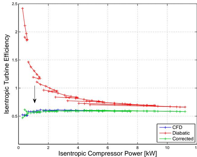
**Figure 1.** Turbine isentropic efficiency
