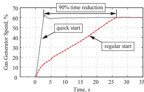
Figure 1: Ground idle start times of a regular engine start [4]
