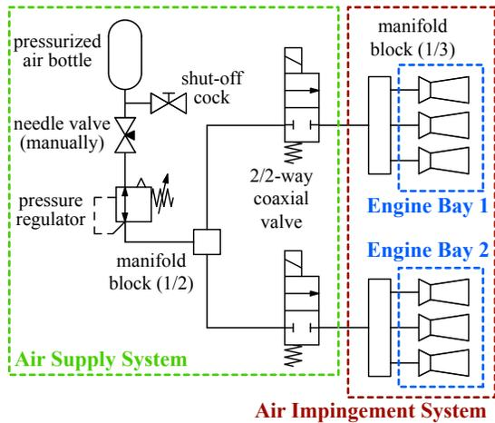
**Figure 3:** Scheme of an airworthy quick-start system for testbed application and helicopter integration
