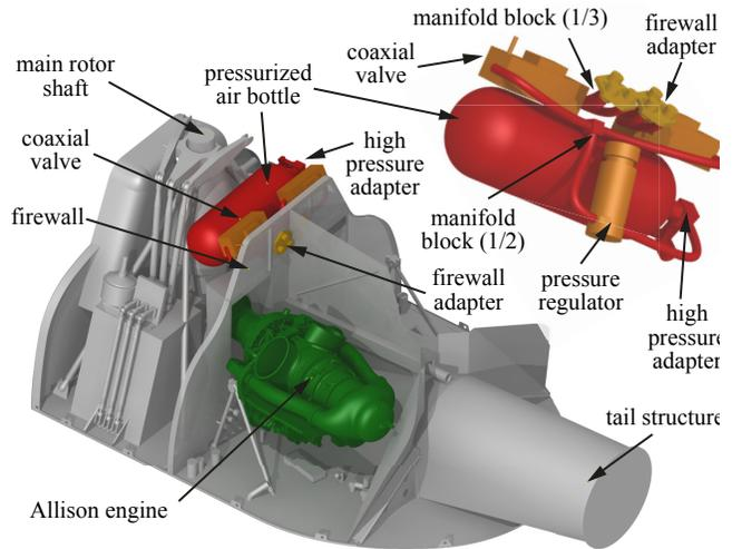
**Figure 4:** CAD model of a possible QSS arrangement within the BO 105 fuselage
