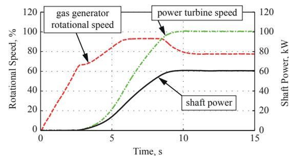
Figure 2: Power delivery curve after performing a quick-start to flight mode start. [4]
