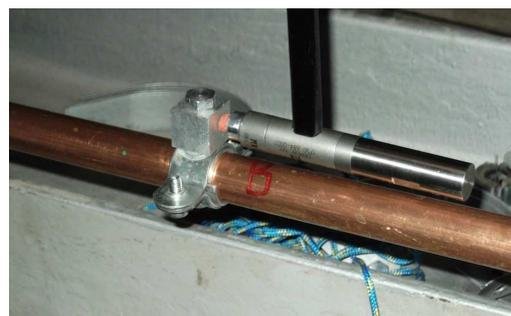
**Figure 5.** Modal hammer with elastic tip used for generating pipeline transient vibrations
