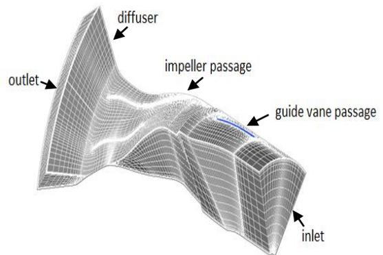
**Figure 2 Computational grids of the compressor**
