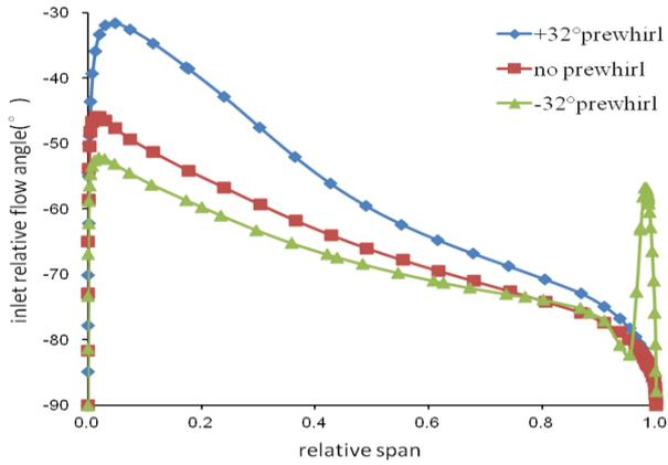
**Figure 6 Impeller inlet relative flow angle distributions at 50,000rpm and mass flow rate 0.36**
