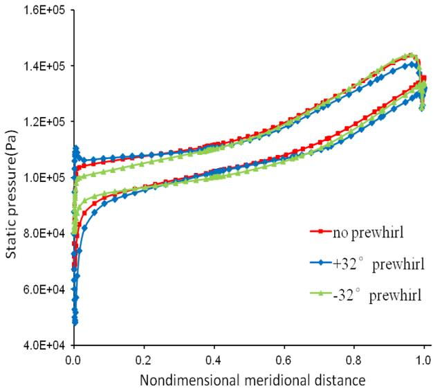
**Figure 9 Blade loading at 90% span, 50,000rpm and mass flow rate of 0.36**
