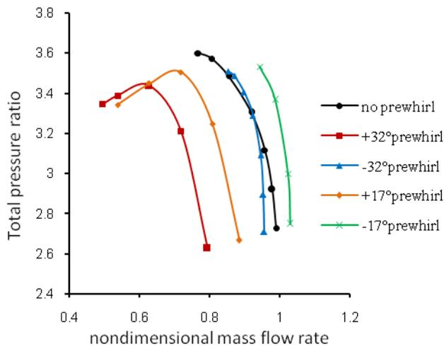
(c) Pressure characteristic at 80,000rpm
