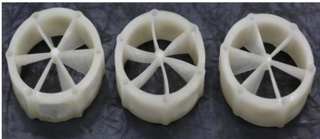
**Figure 19** Photos of the inlet guide vane prototypes (from left to right: positive preswirl vane, twisted guide vane and negative preswirl vane)
