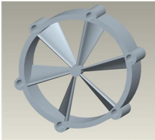
**Figure 3** CAD model of inlet guide vanes
