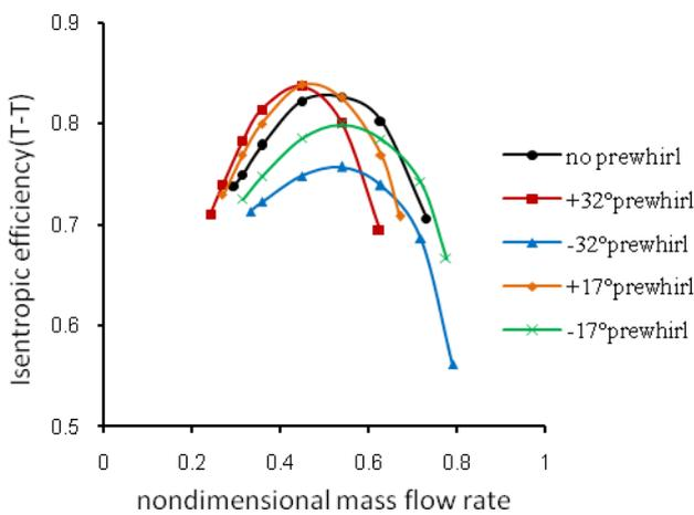
(b) Efficiency characteristic at 50,000rpm
