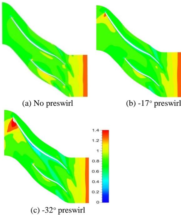
**Figure 12 Relative Mach number contour at 90% span, 50,000rpm and mass flow rate of 0.72**
