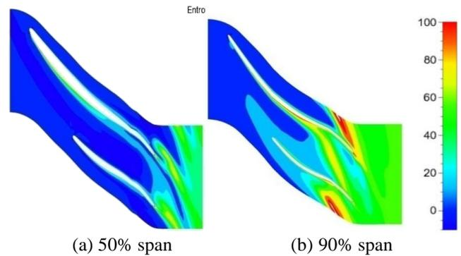
**Figure 14 Entropy contour with  $-17^\circ$  preswirl at 50,000rpm and mass flow rate of 0.72**
