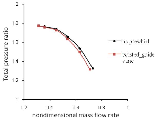
(a) Pressure characteristic at 50,000rpm
