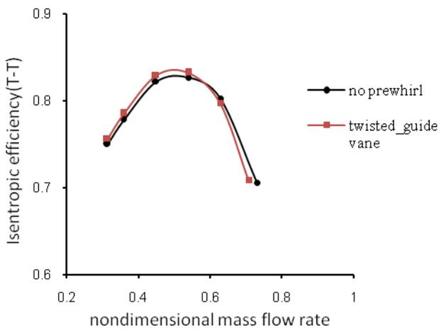
(b) Efficiency characteristic at 50,000rpm
