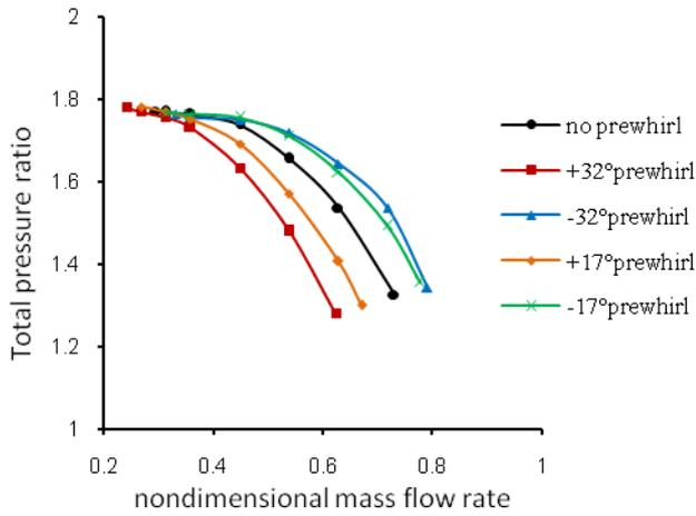
(a) Pressure characteristic at 50,000rpm
