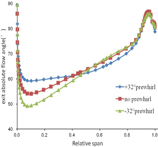
**Figure 10 Impeller exit absolute flow angle distributions at 50,000rpm and mass flow rate of 0.36**
