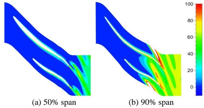
**Figure 13 Entropy contour with no preswirl at 50,000rpm and mass flow rate of 0.72**
