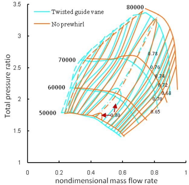
**Figure 22 Performance characteristics of twisted guide vane and no preswirl.**
