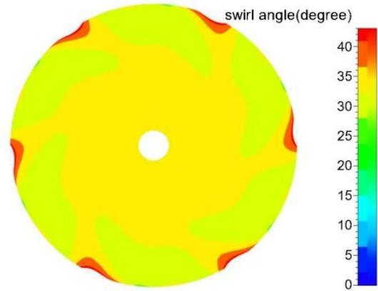
**Figure 4** Swirl angle at vane exit, vane case 3,  $+32^\circ$  mean swirl
