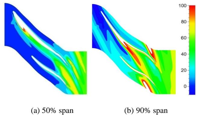
**Figure 15 Entropy contour with  $-32^\circ$  preswirl at 50,000rpm and mass flow rate of 0.72**
