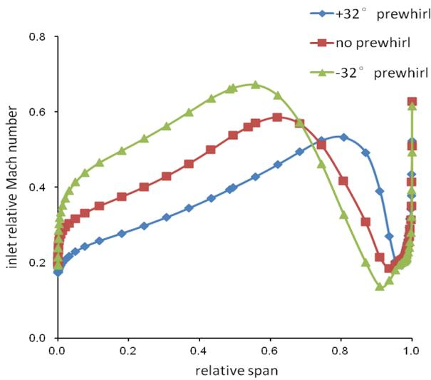
**Figure 7 Impeller inlet relative Mach number distributions at 50,000rpm and mass flow rate 0.36**
