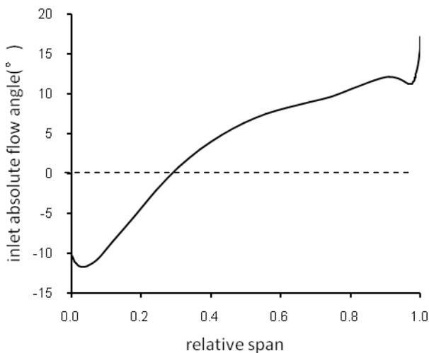
**Figure 17 Impeller inlet absolute flow angle distribution at mass flow rate 0.54, twisted guide vanes**
