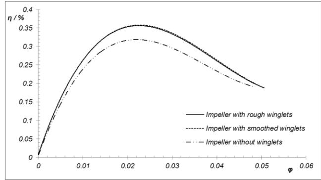
Figure 10. Efficiency over flow coefficient for study 2
