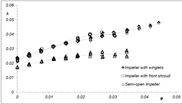
Figure 8. Power coefficient over flow coefficient for study 1
