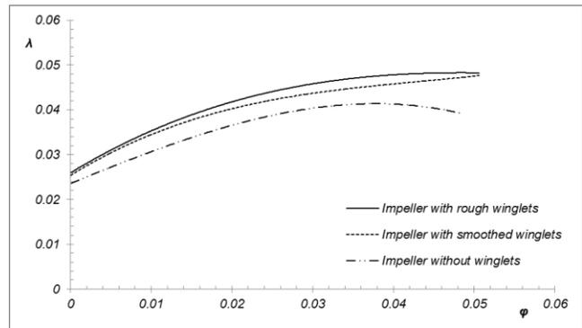
Figure 11. Power coefficient over flow coefficient for study 2
