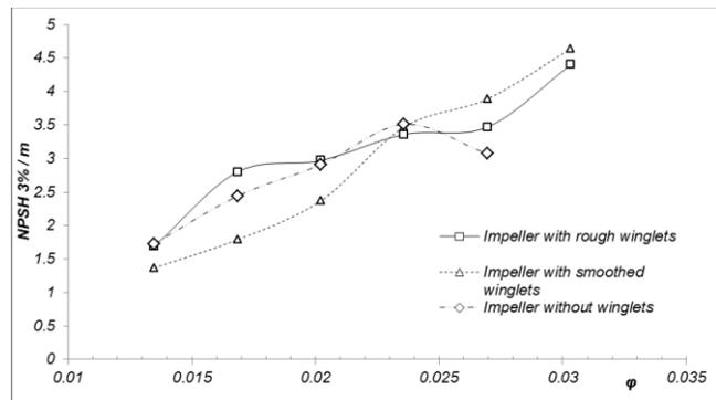
Figure 12. NPSH<sub>3%</sub> over flow coefficient for study 2
