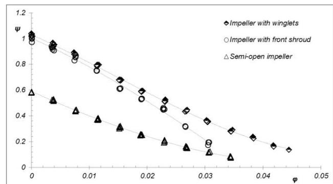
**Figure 6.** Pressure coefficient over flow coefficient for study 1
