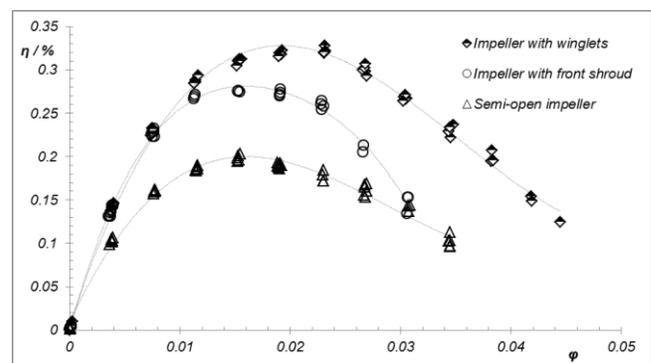
**Figure 7.** Efficiency over flow coefficient for study 1
