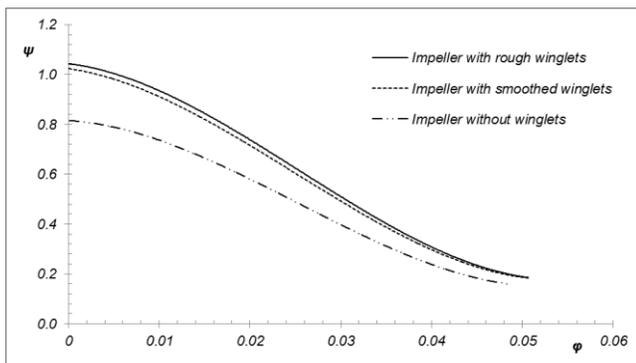
Figure 9. Pressure coefficient over flow coefficient for study 2
