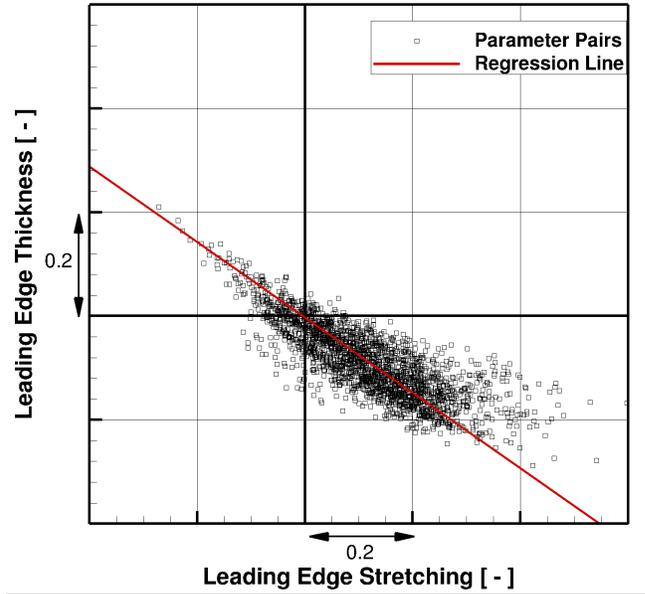
Figure 5. Correlations between leading edge stretching and thickness at front stage rotor
