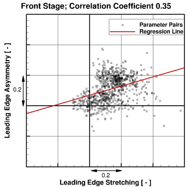
**Figure 9.** Correlations between leading edge stretching and asymmetry at front stage stator
