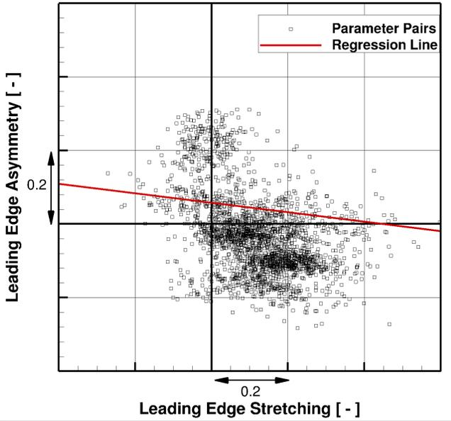
Figure 4. Correlations between leading edge stretching and asymmetry at front stage rotor
