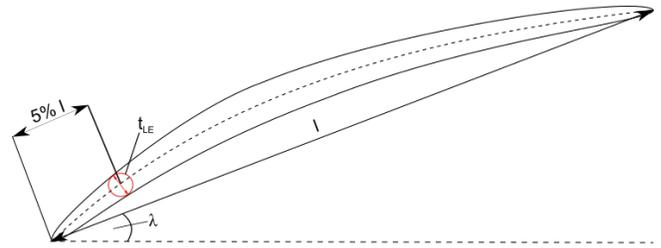
**Figure 3.** Definition of leading edge thickness
