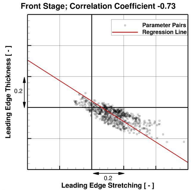
**Figure 10.** Correlations between leading edge stretching and thickness at front stage stator
