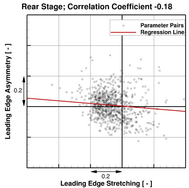
**Figure 11.** Correlations between leading edge stretching and asymmetry at rear stage stator
