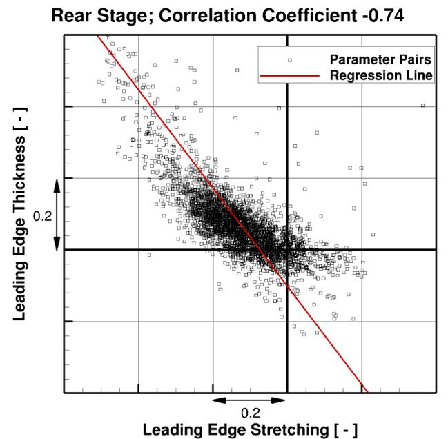
**Figure 8.** Correlations between leading edge stretching and thickness at rear stage rotor
