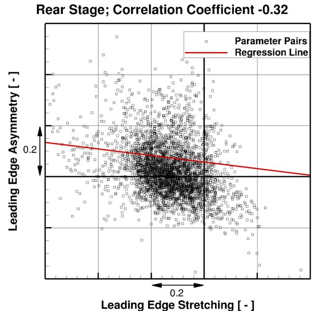
**Figure 7.** Correlations between leading edge stretching and asymmetry at rear stage rotor
