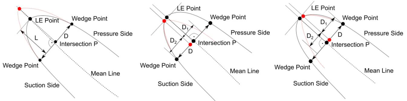
**Figure 2.** Definition of stretching and edge asymmetry caused by erosion on pressure and suction side
