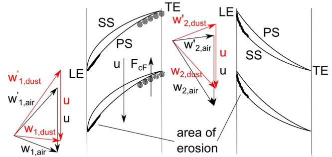
Figure 6. Velocity triangles for air and dust particles
