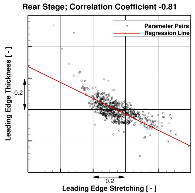
**Figure 12.** Correlations between leading edge stretching and thickness at rear stage stator
