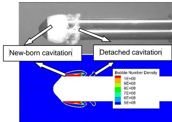
Figure 11 The collapse of the detached cavitation.
