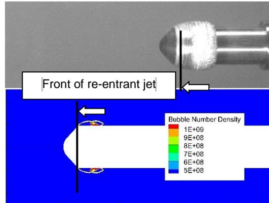
Figure 8 The development of the re-entrant jet.
