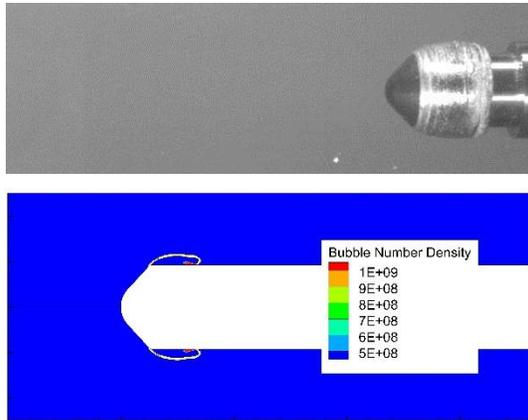
Figure 7 The growth of the sheet cavitation
