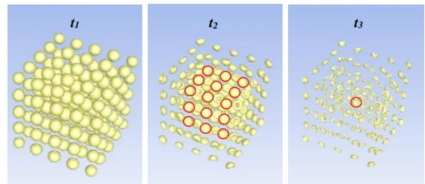
Figure 3 Collapse of bubble cluster ( $\alpha = 0.150, N=5^3, p' = 0.8$ )
