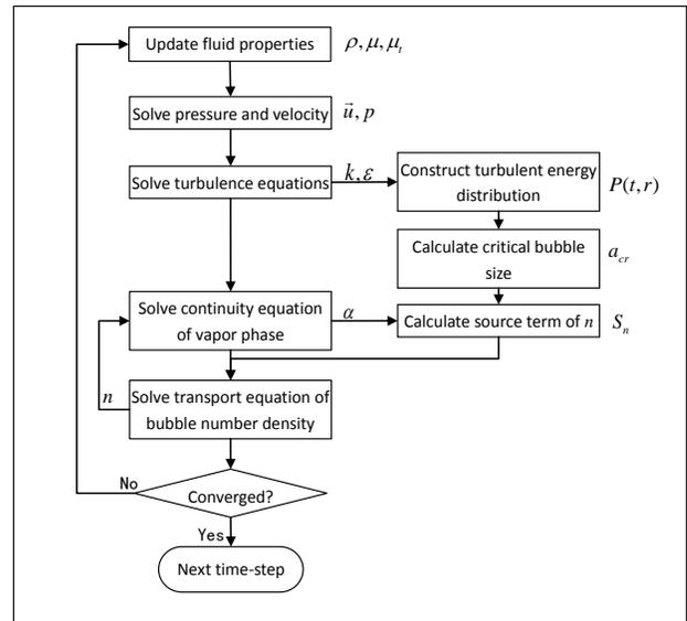
Figure 5 Numerical procedure.
