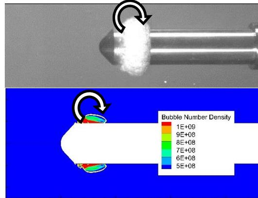
Figure 10 The detachment of cloud cavitation.
