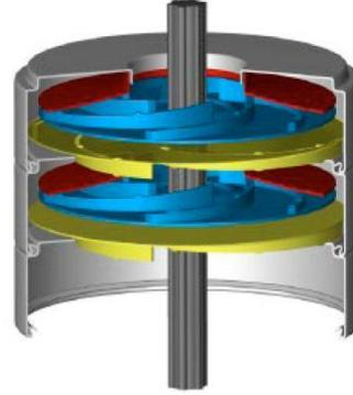
**Figure 1.** Two stages of the investigated centrifugal pump
