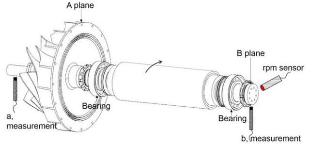
**Figure 3.** Indicated correction planes and vibration measurement points for balancing.
