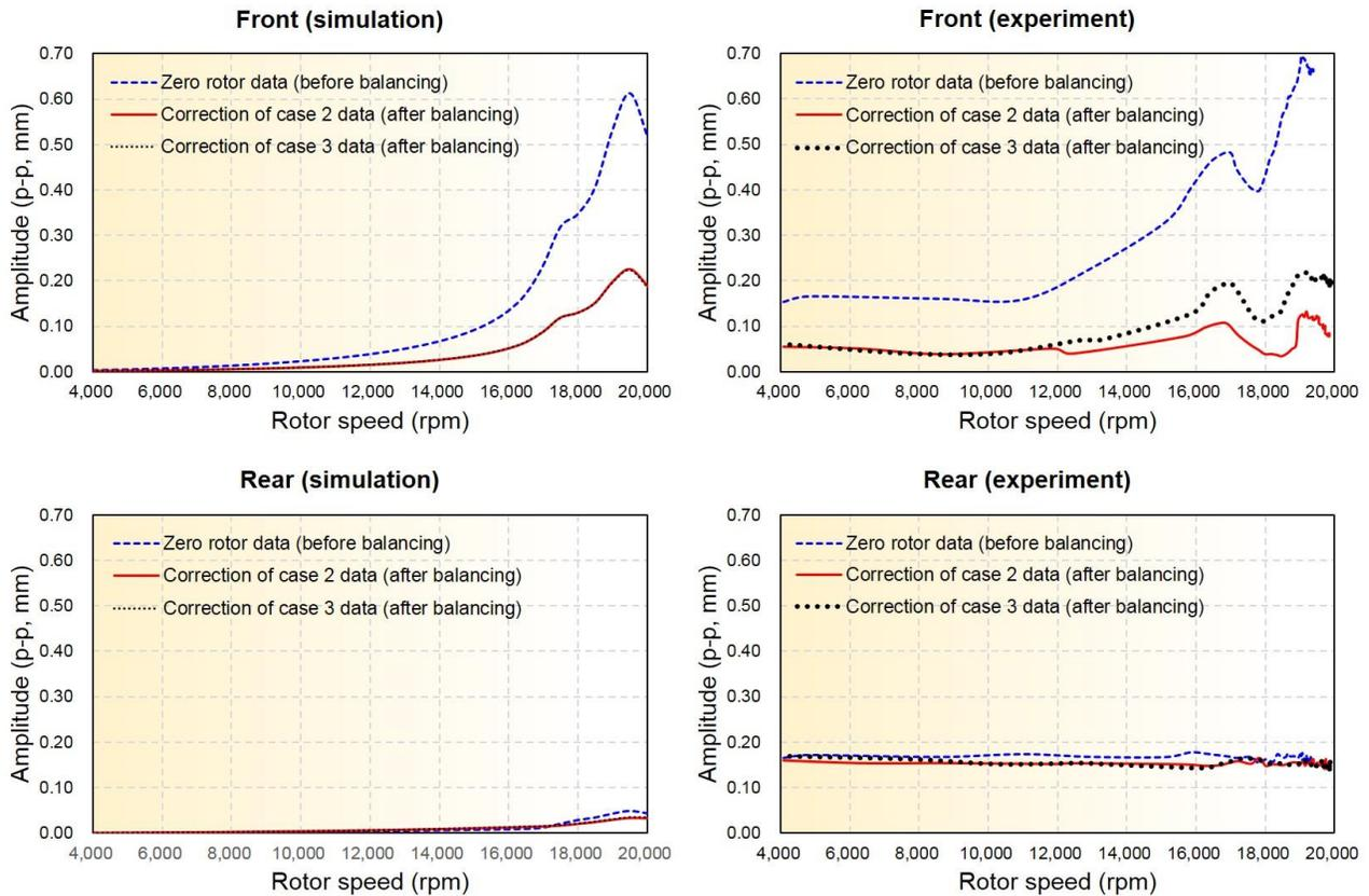
Figure 6. Comparison of simulation and experimental results with balancing (during the speed-up).
