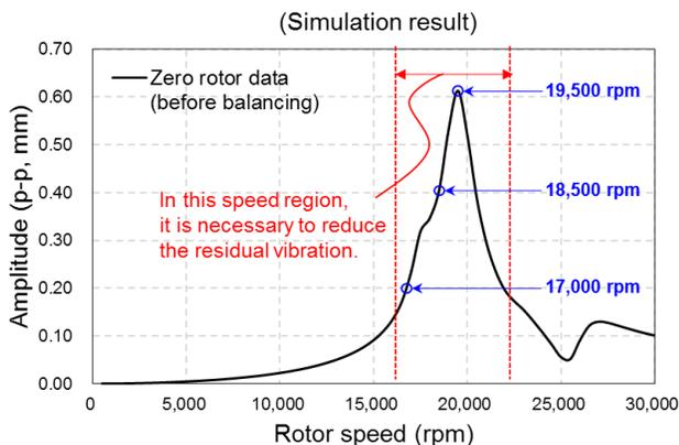
Figure 5. Imbalance response simulation result at 'a' plane.
