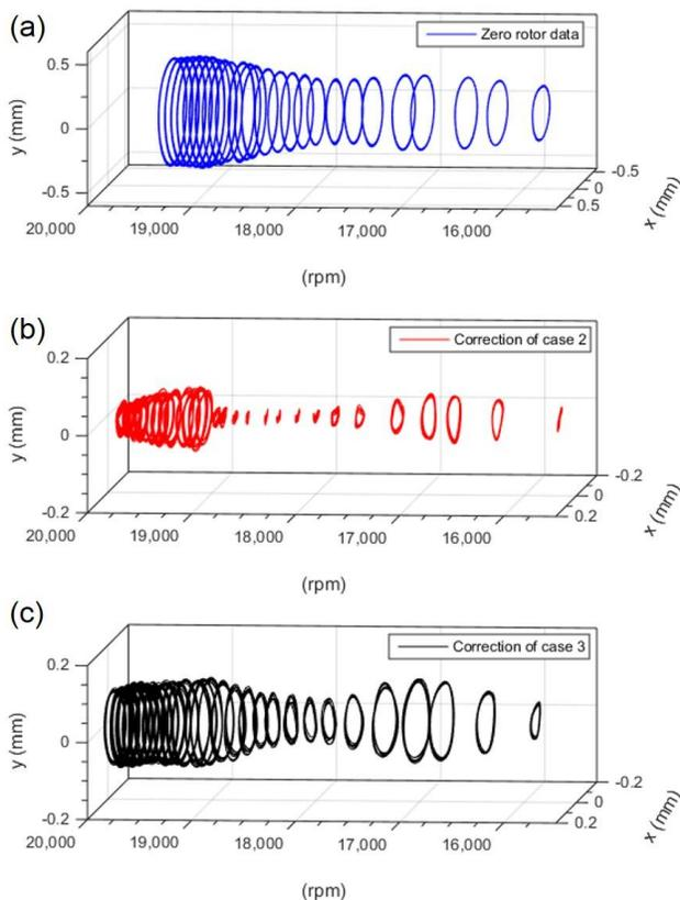
Figure 7. Orbital vibrations in impeller side during the rotor speed-down: (a) zero rotor data, (b) correction of case 2 and (c) correction of case 3.
