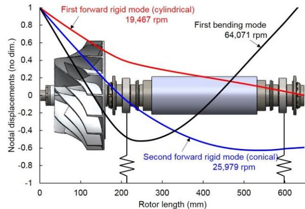
Figure 1. Rigid rotor and mode shape analysis results.
