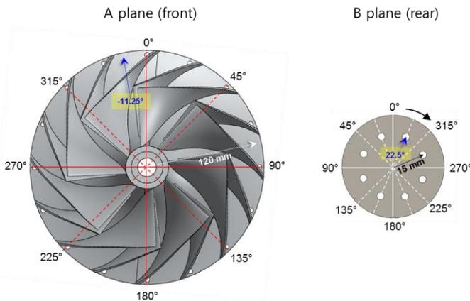
Figure 4. Schematic view of correction A and B plane.
