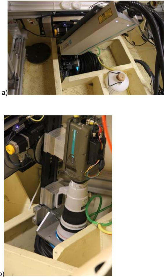
**Figure 8.** Applied measurement hardware on the “Amandine” mounted on a linear and rotary stage to the porthole
