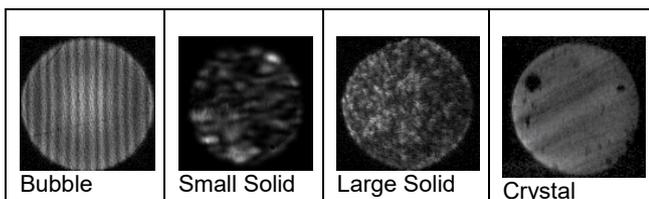
**Figure 3.** Interference pattern of different particle types
