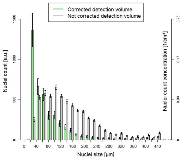
**Figure 10.** Particle size and particle count concentration distribution for the measurement on the “Amandine” with error bars.
