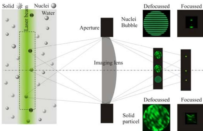
**Figure 2** Principle of the HDNC technique [7]
