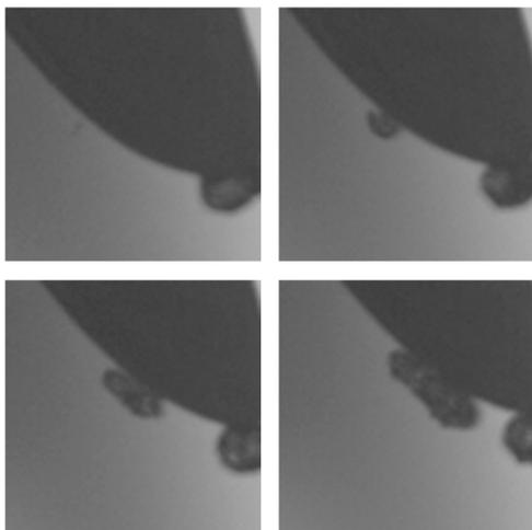
**Figure 1.** A bubble expanding at propellers surface recorded with a high speed camera and stroboscopic illumination
