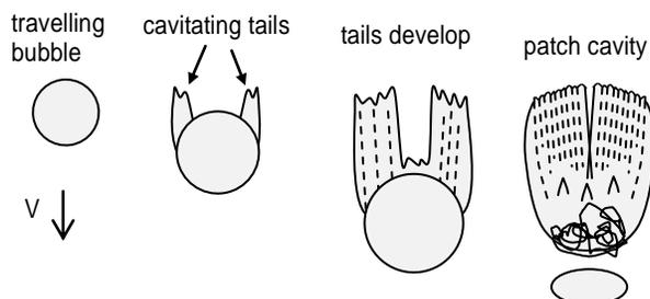
**Figure 7.** Inception process for a travelling bubble and a laminar boundary layer based on [10, 36], flow  $V$  from top to bottom.
