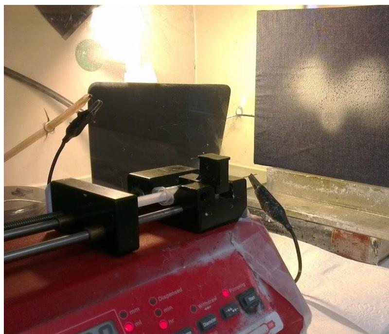
**Figure 8.** Deposition of PU nanofibers on denim fabric surface
