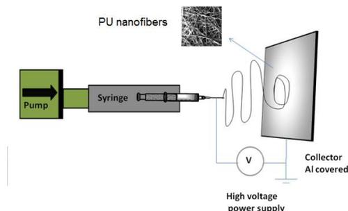
**Figure 3.** Schematic illustration of the nanofiber electrospinning process
