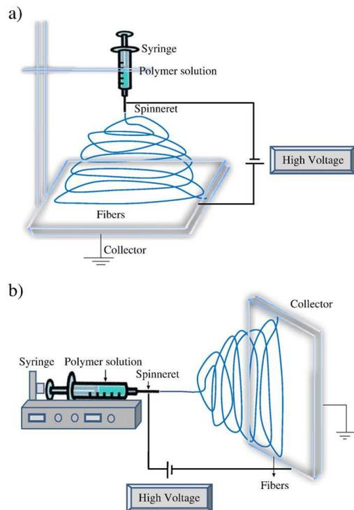
**Figure 2.** Schematic diagram of set-up of electrospinning
