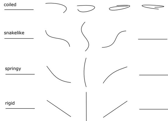
**Figure 3.** Sketch of four different orbit types of fibres in shear flow: rigid, springy, snakelike and coiled [8],[11].
