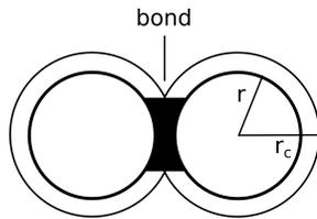
**Figure 1.** The particle radius,  $r$ , and the contact radius  $r_c$  is defined when modeling bonded particles. Bonds are formed if there is particle contact within the radius  $r_c$ . Bond properties include normal and shear stiffness of the bond and critical shear and normal stress break criteria.
