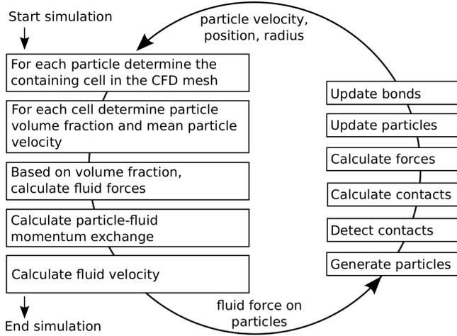
**Figure 4.** Block diagram of calculation process in a coupled CFD-DEM simulation. The blocks to the left represent the CFD solver and the blocks to the right represent the DEM solver.
