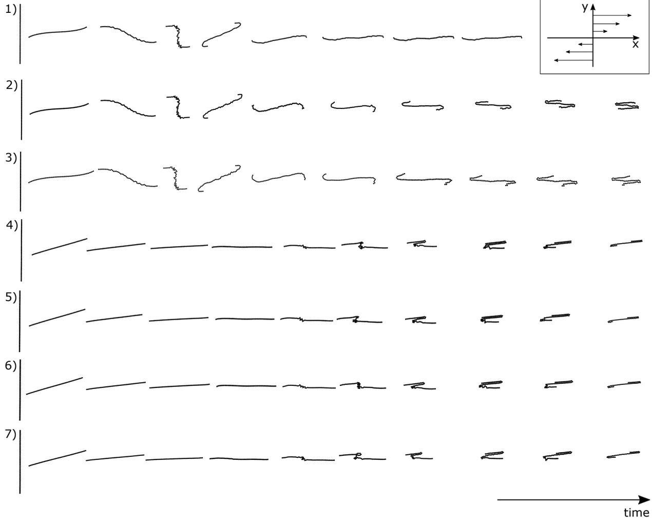
**Figure 6.** Development of the fiber shape with time in the different cases. The time interval between each image in a case is 1 s.
