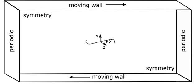
**Figure 5.** CFD domain. The upper and lower boundaries are moving walls with no slip. This creates a shear flow in the domain. The right and left part of the domain has periodic boundary conditions. The fiber of DEM particles orbits in the center of the domain.
