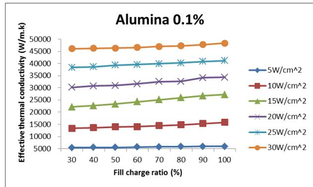
Figure 3. Effective thermal conductivity of the heat pipe versus fill charge ratio
