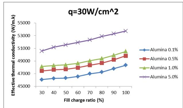
Figure 10. Effective thermal conductivity of the heat pipe versus fill charge ratio
