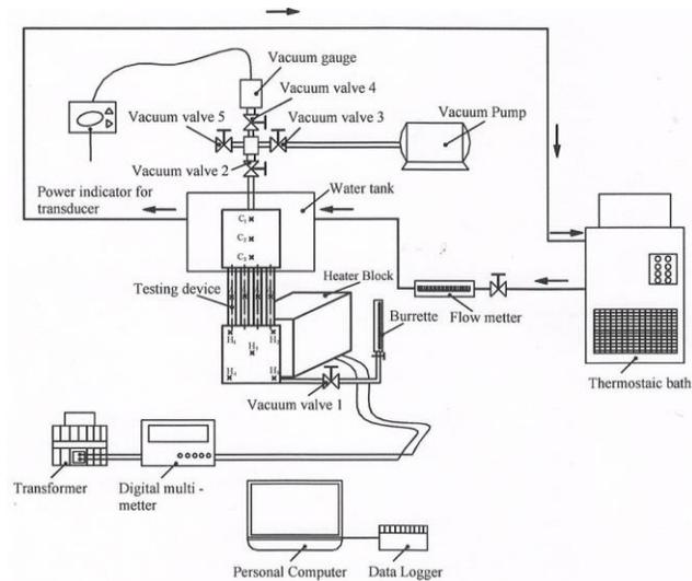
Figure 1. Schematic design of the experimental apparatus
