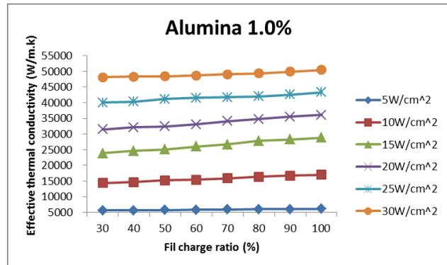
Figure 5. Effective thermal conductivity of the heat pipe versus fill charge ratio
