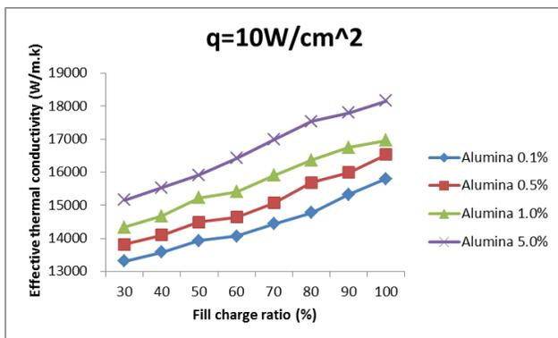
Figure 8. Effective thermal conductivity of the heat pipe versus fill charge ratio
