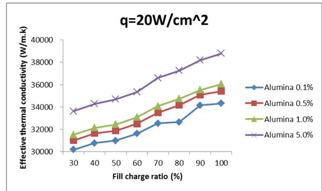
Figure 9. Effective thermal conductivity of the heat pipe versus fill charge ratio
