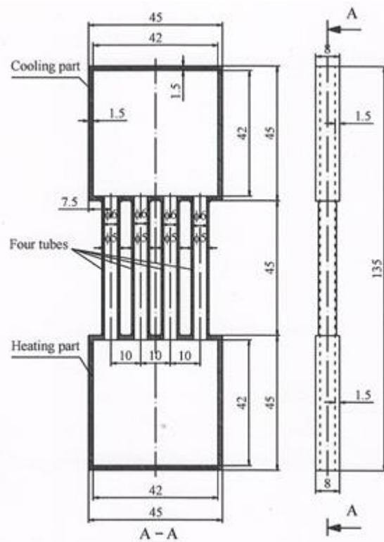
Figure 2. Structure of self oscillating multi heat pipe (unit inmm)
