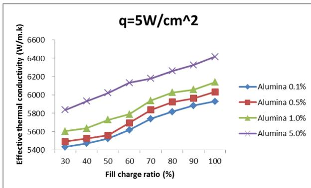
Figure 7. Effective thermal conductivity of the heat pipe versus fill charge ratio
