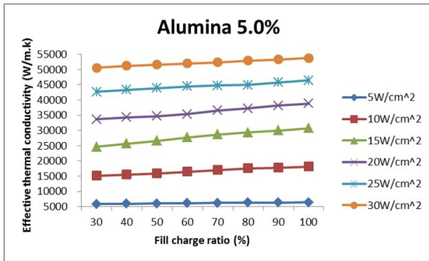
Figure 6: Effective thermal conductivity of the heat pipe versus fill charge ratio
