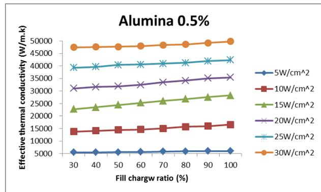
Figure 4. Effective thermal conductivity of the heat pipe versus fill charge ratio
