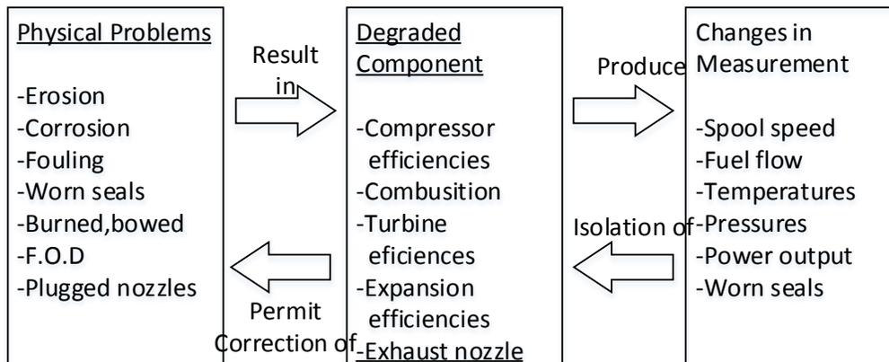
Figure 1. Gas turbine fault diagnostics approach
