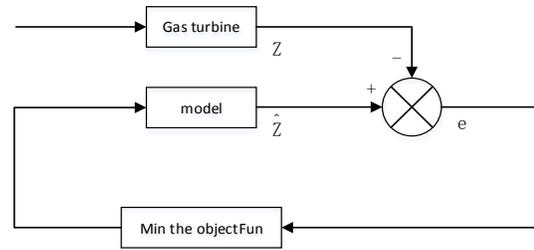
Figure 2. Model based gas turbine fault diagnostics
