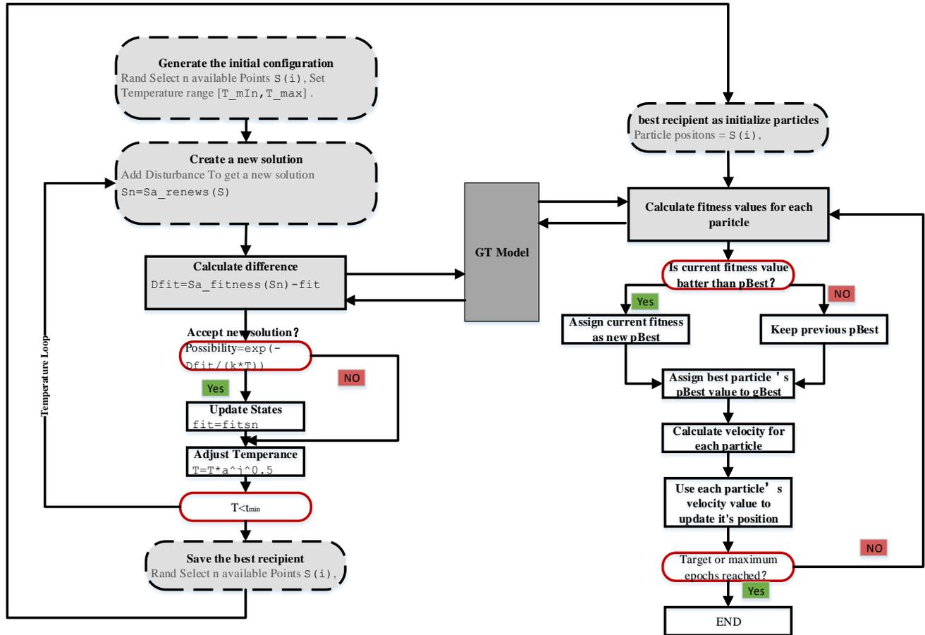
Figure 3. Fault diagnostic procedure of SA-PSO method
