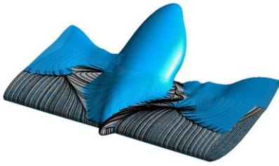
**Figure 8.** Limiting streamlines and recirculation regions shown by isosurface of zero longitudinal velocity (SST  $k-\omega$ , modified airfoil,  $15^\circ$ )
