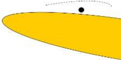
**Figure 16** Sketch of a bubble (the filled circle) in a separation zone near the hydrofoil leading edge (its boundary shown by the dotted line).
