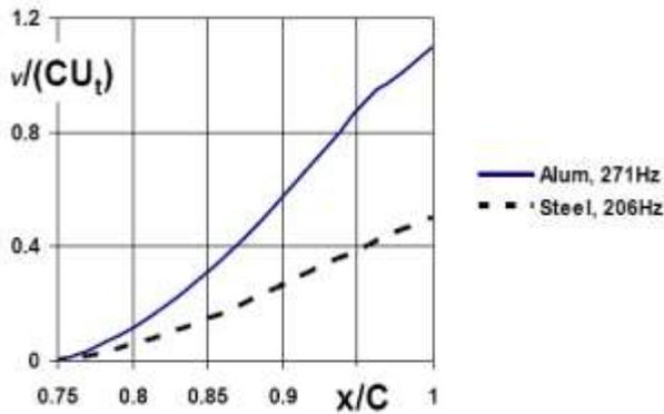
Figure 9 Chordwise bending deformation of the hydrofoil section at resonances
