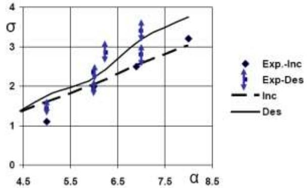
**Figure 18** Computed [16] and measured [7] cavitation inception and desinence numbers for the steady water tunnel flows around Cav2003
