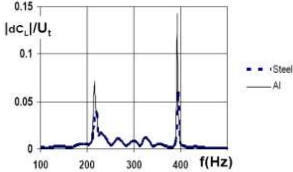
Figure 5 Computed lift pulsation spectra for aluminum and steel hydrofoils Cav2003 in water tunnel
