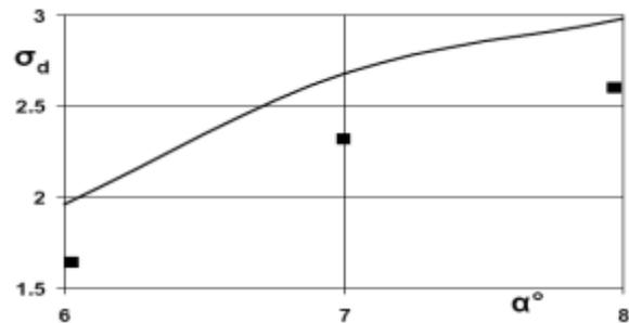
**Figure 19** Comparison of computed (line) and measured [6] cavitation desinence number for the steel hydrofoil.
