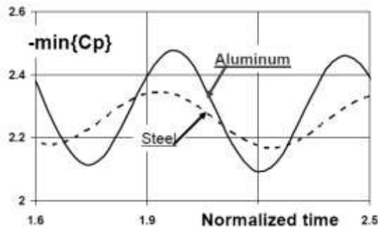
Figure 13 Histories of  $C_p$  minima at  $\alpha=6^\circ$  for hydrofoils made from different materials.
