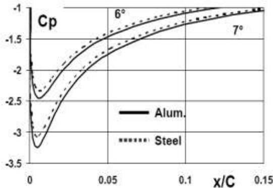
Figure 12 Pressure distributions near leading edges of hydrofoils made from different materials
