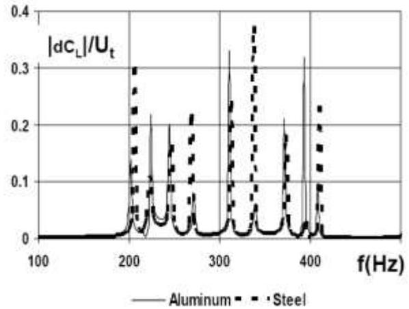
Figure 11 Impact of material on lift coefficient pulsation of tip section of hydrofoil Cav2003 in a water tunnel
