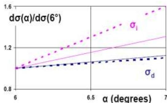
**Figure 20** Hydrofoil material impact on  $\sigma_d$  and  $\sigma_i$ ; dashed lines show data [6], solid – numerical results
