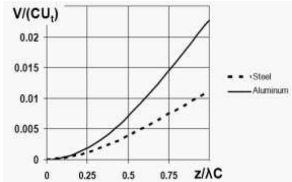
Figure 7 Hydrofoil spanwise bending deformations at bending resonances
