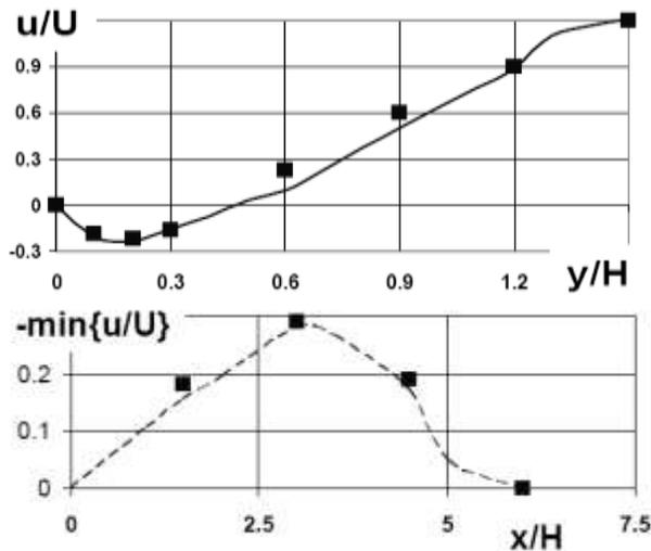
**Figure 17** Computed (lines) and measured velocities across (in the top, with data [19]) and along (in the bottom, with data [20]) separation zones.
