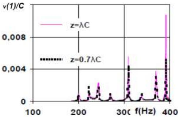
Figure 8 Deflection of trailing edges of diverse sections of the aluminum Cav2003 in the water tunnel
