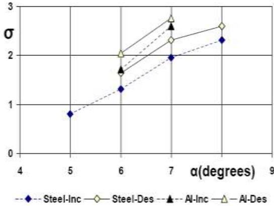
**Figure 3** Observed [6] cavitation inception and desinence numbers for aluminum and steel Cav2003
