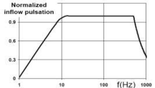
**Figure 4** Excitation spectra for a water tunnel normalized by the maximum harmonic
