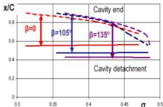
Figure 2 Computed cavity detachments (solid lines) and ends (dashed lines) on hydrofoils Cav2003 for  $C_L=0.125$  at the flow speed 10m/s;  $\beta=0$  corresponds to hydrophilic surface (metals), other  $\beta$  correspond to hydrophobic surface (as Teflon).
