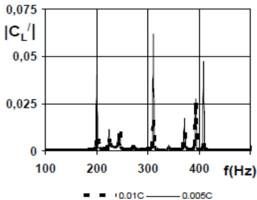
Figure 10 Example of the impact of trailing edge thickness on lift coefficient pulsation of the tip section of aluminum hydrofoil Cav2003 in the water tunnel
