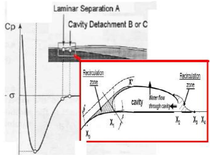
Figure14 Sketch of an attached cavity
