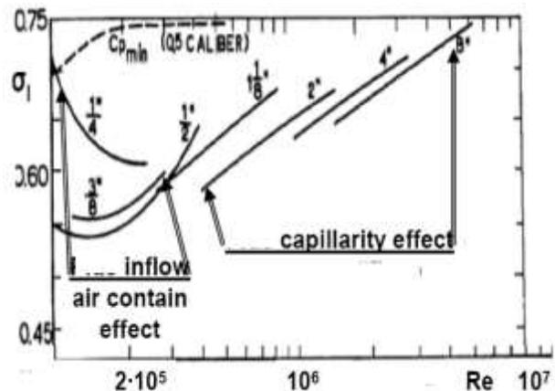
Figure 15 Experimental dependencies of cavitation inception number on  $Re$  for axisymmetric bodies with hemi-spherical heads; numbers show body diameters  $D$
