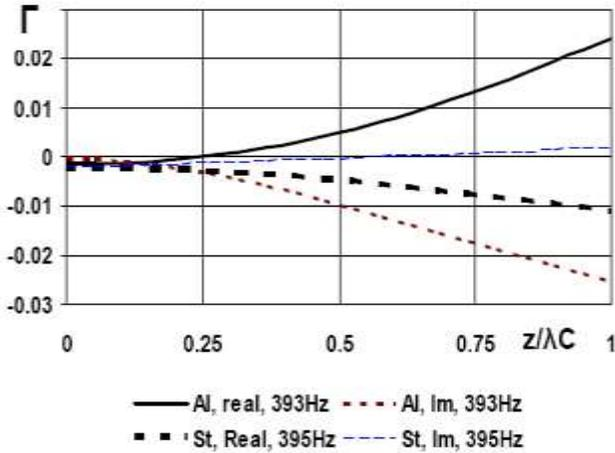
Figure 6 Effect of material on spanwise load distributions on Cav2003 at resonances in a water tunnel
