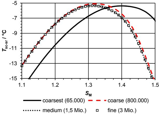
Figure 4a. Mesh independence study – sub-cooling in an extract of the impeller flow channel
