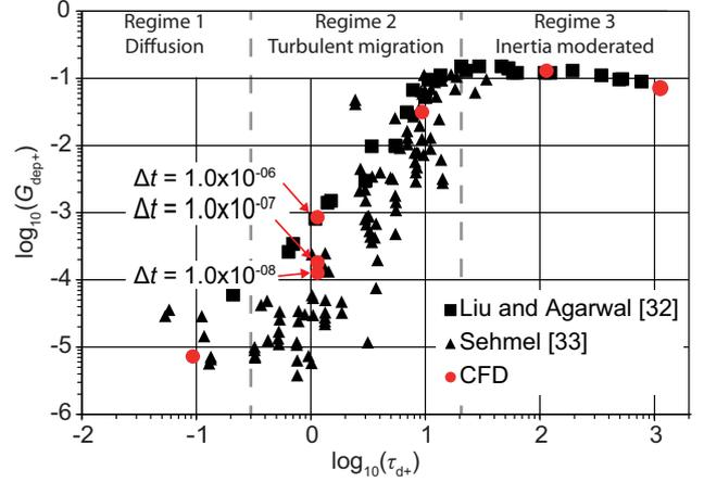
Figure 1. Deposition rate (Eq. 4) in a straight tube as a function of the non-dimensional relaxation time (Eq. 5)
