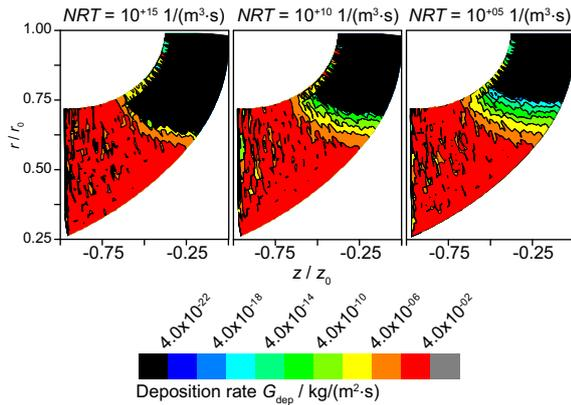
Figure 9. Deposition rate on the blade pressure side
