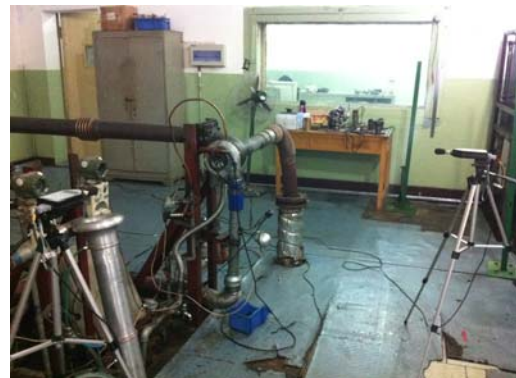
Figure 3. Far field noise measurement setup
