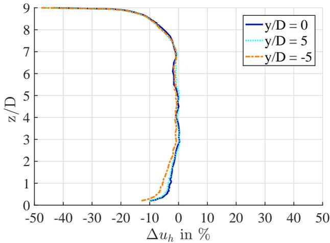
**Figure 7.** Velocity deviations over the channel height for the centerline ( $y/D = 0$ ) and  $y/D = \pm 5$
