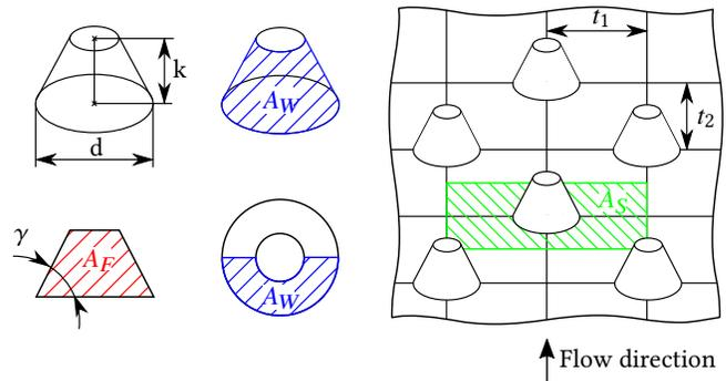
**Figure 3.** Generic test plate surface roughness consisting of truncated cones
