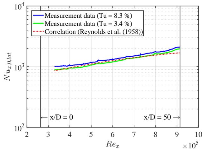
**Figure 11.** Laterally averaged Nusselt numbers without film cooling  $Nu_{x,0}$  against Reynolds number  $Re_x$  for the hot gas turbulence intensities  $Tu_h = 8.3\%$  and  $3.4\%$ , and for a correlation by Reynolds et al. [25]
