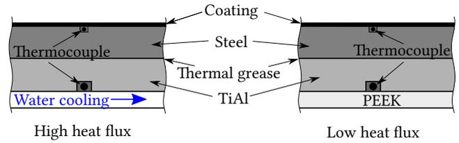
**Figure 6.** Schematic of the test plate configurations for setting two different thermal boundary conditions
