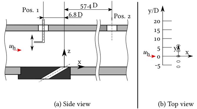
**Figure 4.** Measurement positions for operating point and probe measurements
