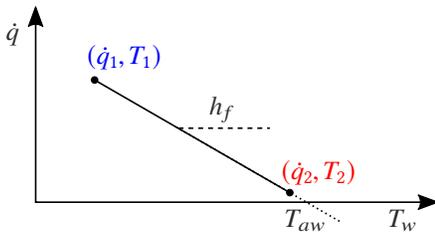
**Figure 5.** Superposition approach to film cooling
