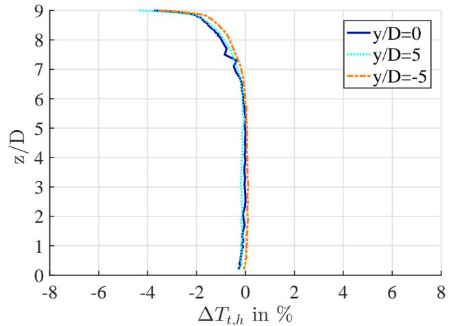
**Figure 9.** Temperature deviations over the channel height for the centerline ( $y/D = 0$ ) and  $y/D = \pm 5$
