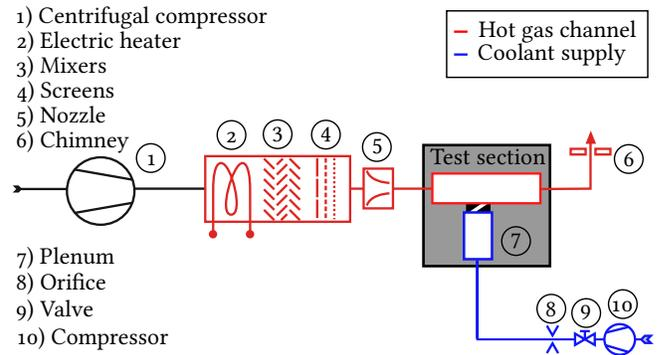
**Figure 1.** Test facility at ITS including hot gas channel and cooling air supply
