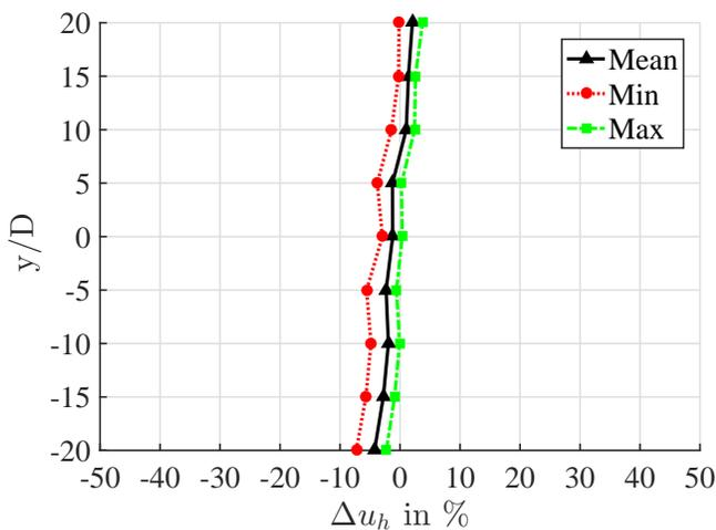
**Figure 8.** Lateral distribution of hot gas flow velocity deviations for  $1 \leq z/D \leq 7$
