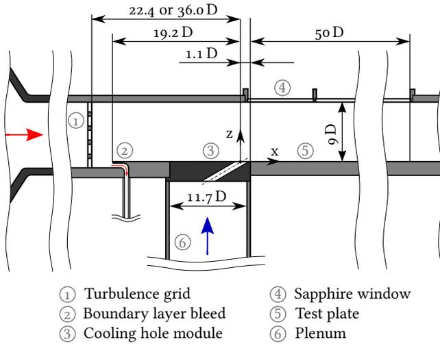
**Figure 2.** Cross-sectional view of the test section
