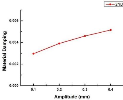
**Figure 2.** Material damping ratio with different amplitude
