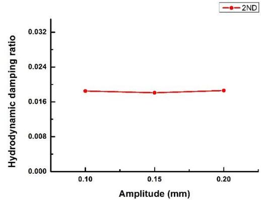
Figure 1. Hydrodynamic damping ratio with different amplitude
