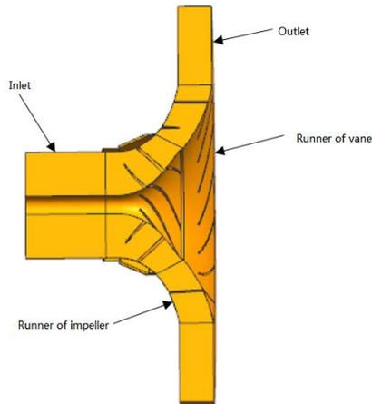
**Figure 8.** Impeller channel model for CFD calculation
