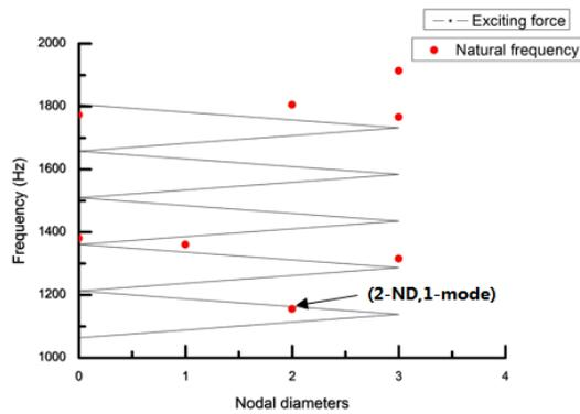
**Figure 9.** Interference diagram of impeller
