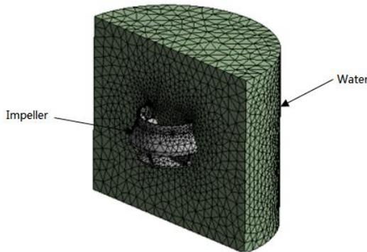
**Figure 7.** FEM model of impeller and water
