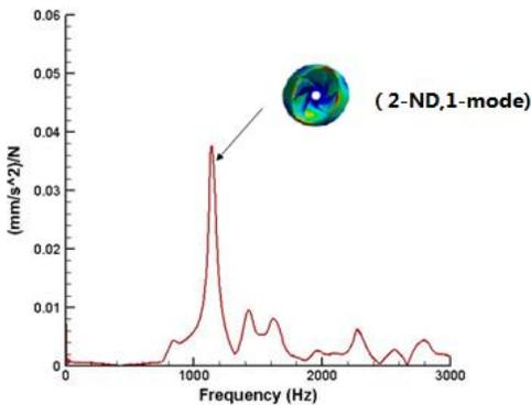
Figure 5. Measured frequency response function
