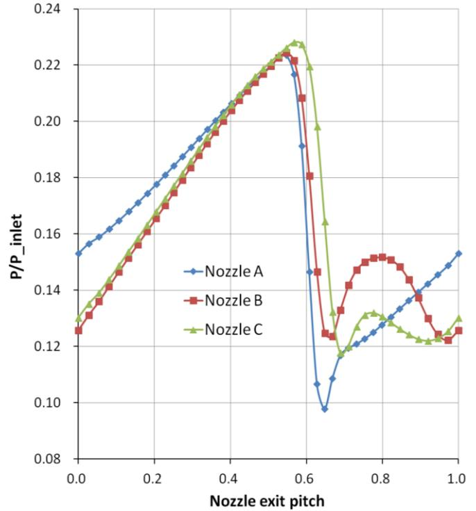
**Fig. 12 Pressure variation at nozzle exit at expansion ratio 6:1, nozzles are closed.**
