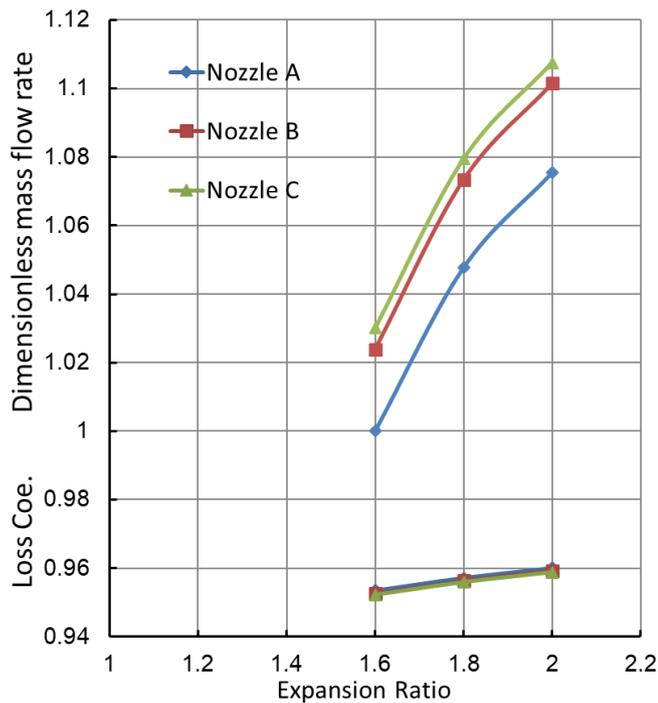
**Fig. 14 Performance of three nozzles in fully opened position**
