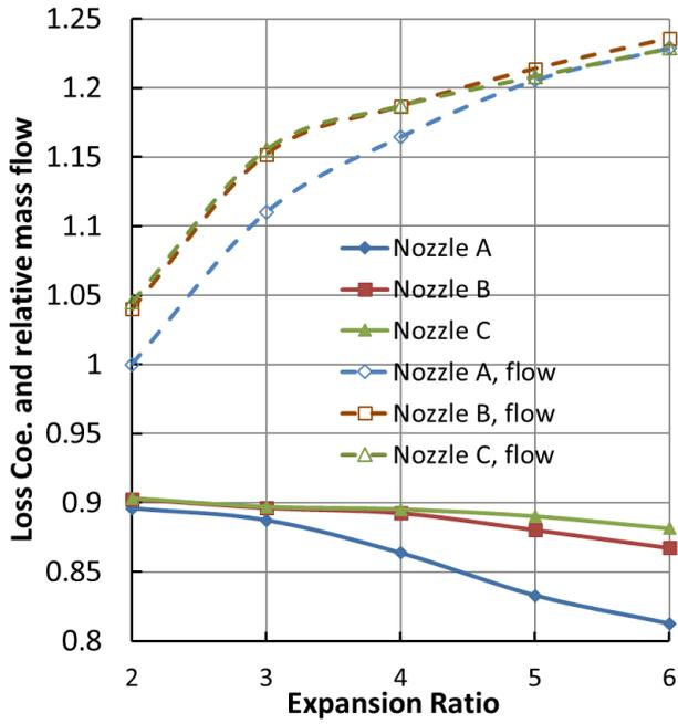
**Fig. 10 Performance of new nozzles at high expansion ratios, nozzles are closed.**
