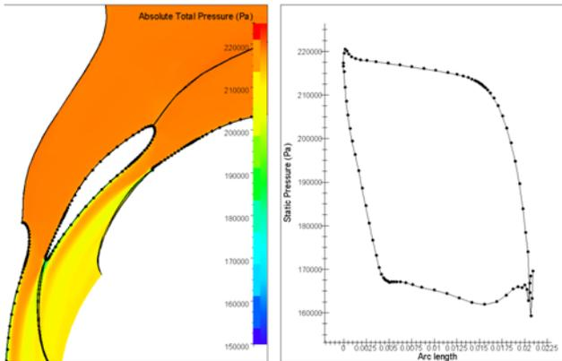
**Fig. 2** Calculated total pressure distribution (left) and static pressure loading (right) of an optimised VNT nozzle
