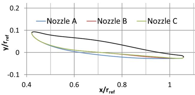
**Fig. 8 Geometry of nozzles A, B and C in the x-y plane**
