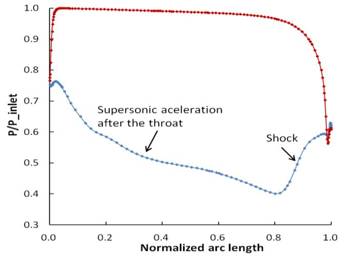
**Fig. 6** Loading of baseline nozzle at 6:1 expansion ratio
