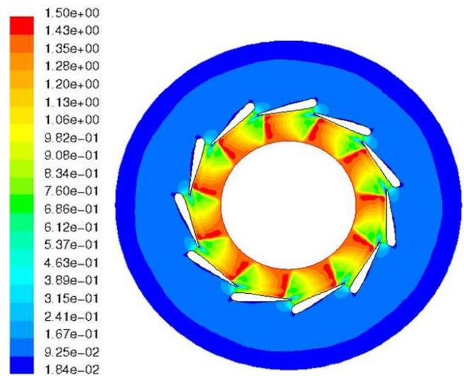
**Fig. 1** Calculated Mach no. of a VNT nozzle ring under a high expansion ratio [1]
