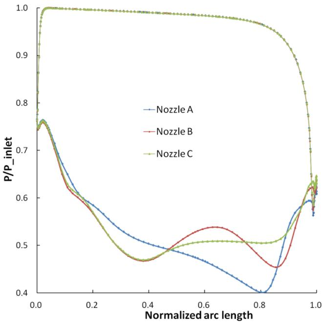
**Fig. 11 Loading of three nozzles at expansion ratio 6:1, nozzles are closed.**
