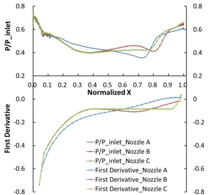
**Fig. 7** Suction surface loading and surface derivative of three different  $x-y$  nozzles. Nozzle A is the mapped baseline. Nozzle expansion ratio = 2:1
