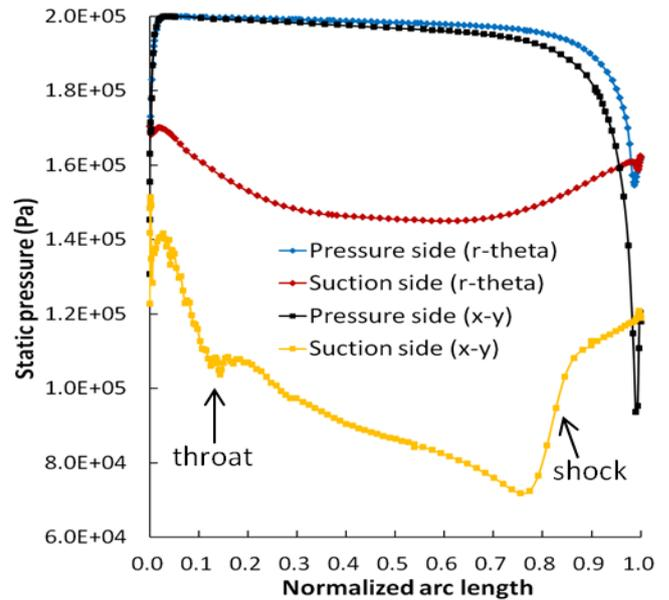
**Fig. 5 Comparison of loading for vanes before and after the conformal mapping, nozzle expansion ratio = 2:1**
