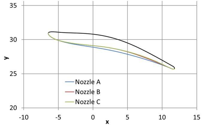
**Fig. 9 Geometry of three nozzles in the r- $\theta$  plane**
