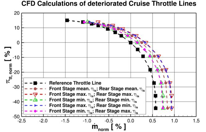
**Figure 5.** CFD-calculations of different deterioration combinations in the HPC
