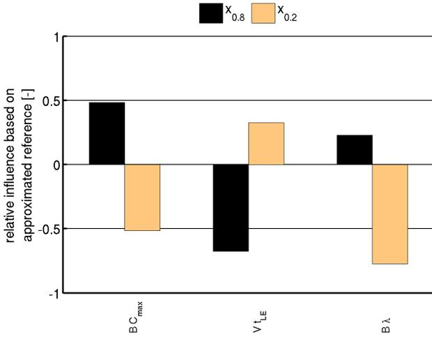
**Figure 4.** Sensitivities of  $\eta_{is}$  to geometric changes at the rear stage
