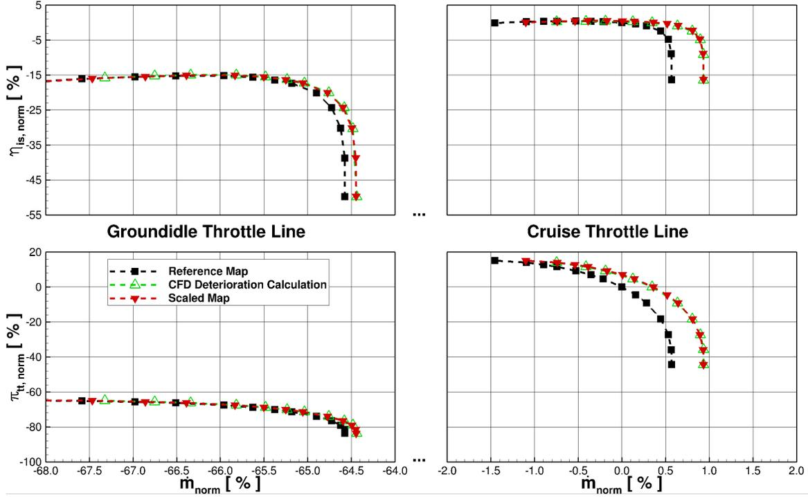
Figure 6. Validation of the HPC map scaling method
