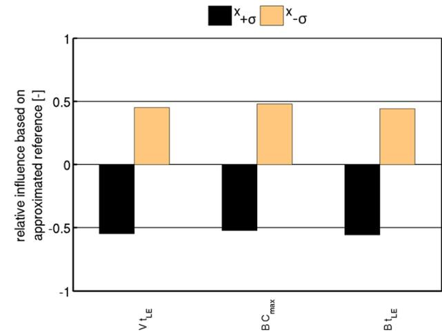
**Figure 2.** Sensitivities of  $\eta_{is}$  to geometric changes at the front stage
