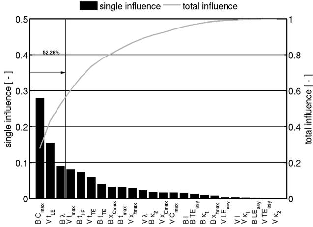
**Figure 3.** Pareto chart of isentropic efficiency  $\eta_{is}$  at the rear stage
