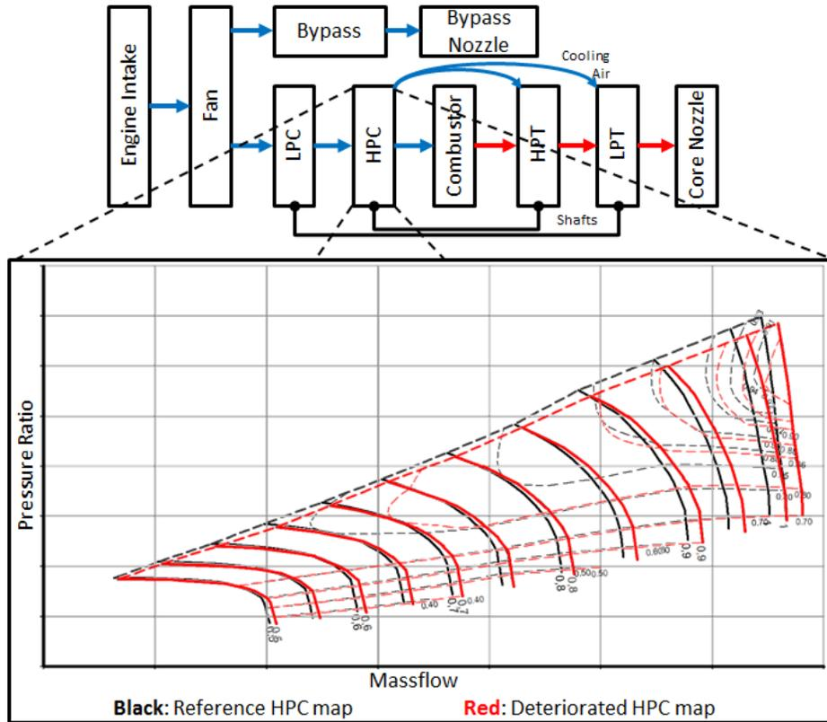
**Figure 7.** Scheme of a modular performance synthesis model with modified HPC maps
