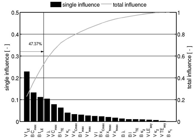
**Figure 1.** *Pareto* chart of isentropic efficiency  $\eta_{is}$  at the front stage
