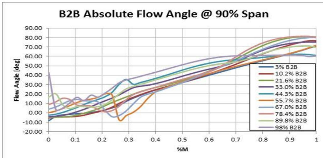
Figure 4. Blade-to-blade flow angle variations taken at the 90% spanwise location; note that these angles cross over each other at 70% distance; at this point, the secondary flow has formed into a tight passage vortex and develops a pattern distinct from the primary flow; impeller at 4° incidence
