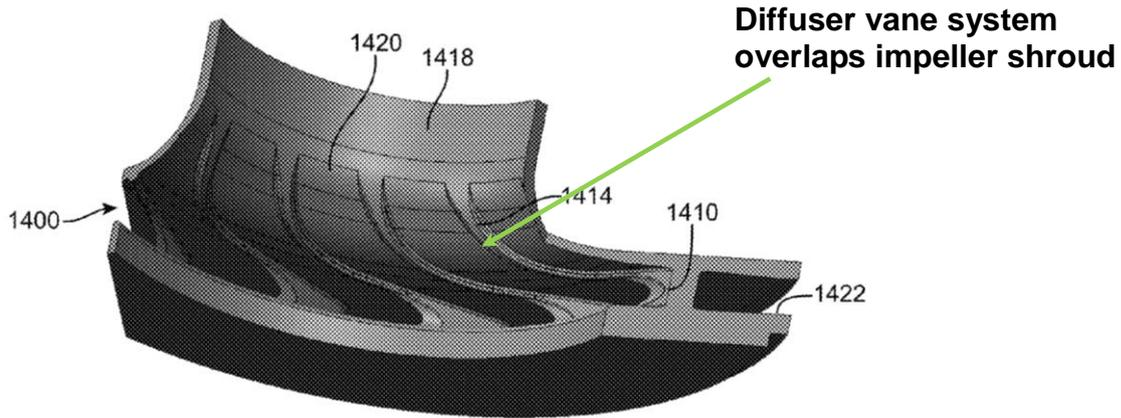
Figure 2. Embodiment of the flow-wise grooved-cover CCFG (Close-Coupled Flow-Guide); Patent 8,926,276
