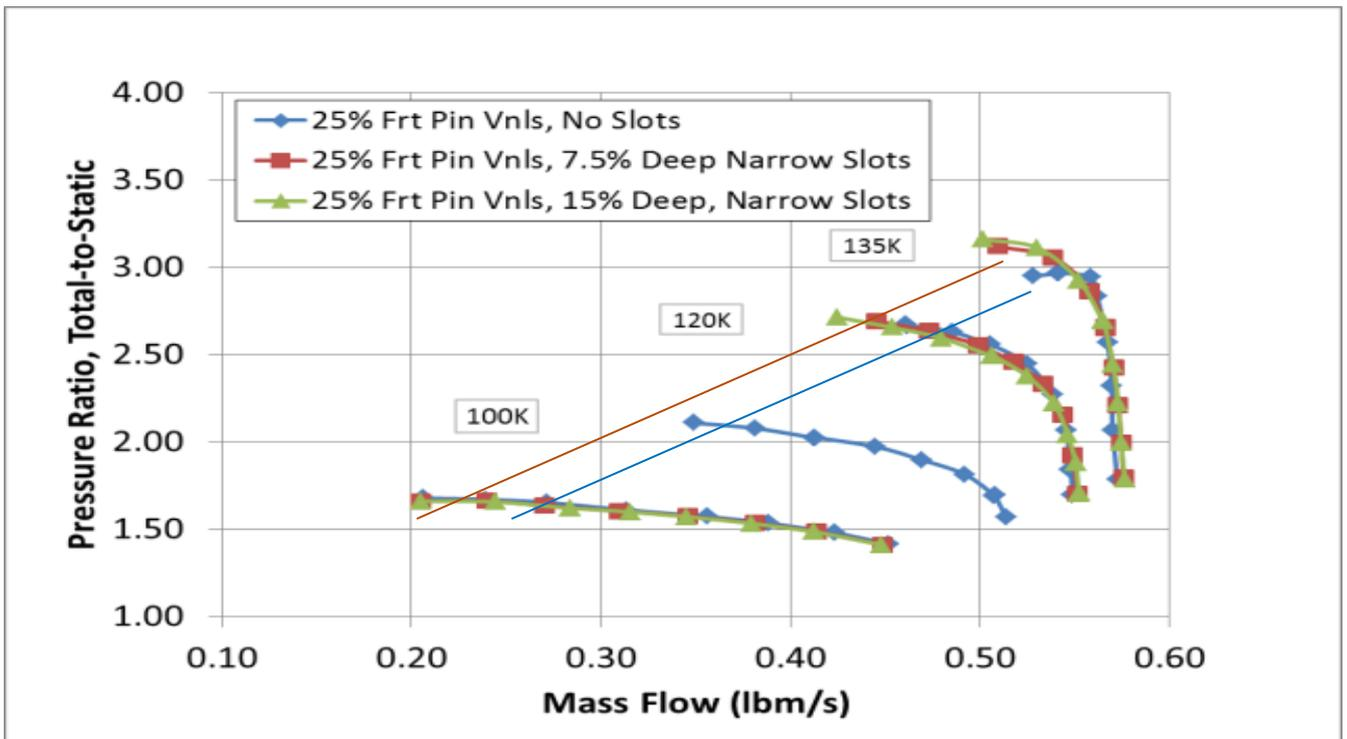
Figure 8a. Pressure Rise for the 7.5% and 15% deep grooves; Figure 6a cover
