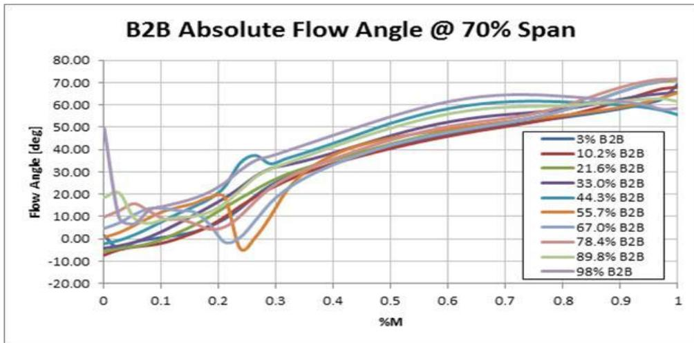
**Figure 5.** Blade-to-blade flow angle variations at the 70% spanwise location; same trends as Figure 4; impeller at 4° incidence
