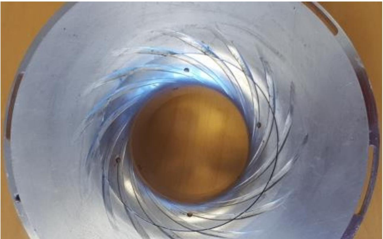
**Figure 6a.** The flow-wise grooved-cover (aka CCFG) showing the impeller cover below the reference circle and outside the circle is the diffuser front plate (25% front pinch configuration); grooves to 30% meridional distance past impeller
