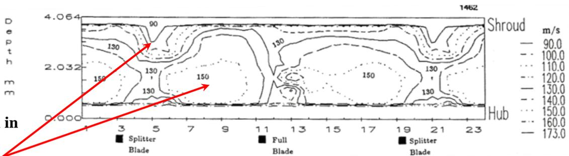
Figure 1a. L2F measurements:  $C_m$ ; near diffuser inlet,  $r = 1.1r_2$ ; 80 krpm, 0.303 lbm/sec
