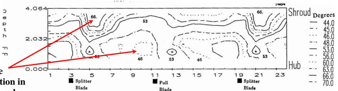
Figure 1c. L2F measurements:  $\alpha$ ; near diffuser inlet,  $r = 1.1r_2$ ; 80 krpm, 0.303 lbm/sec
