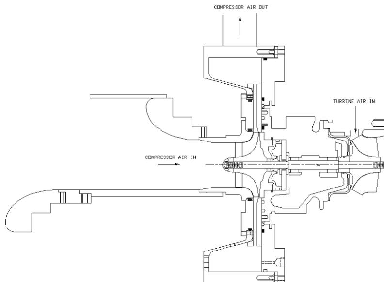
**Figure 7.** 60 mm test rig as used for consortium work; both the short and long inlets are illustrated in this diagram. Four exit ports from the collector are used.
