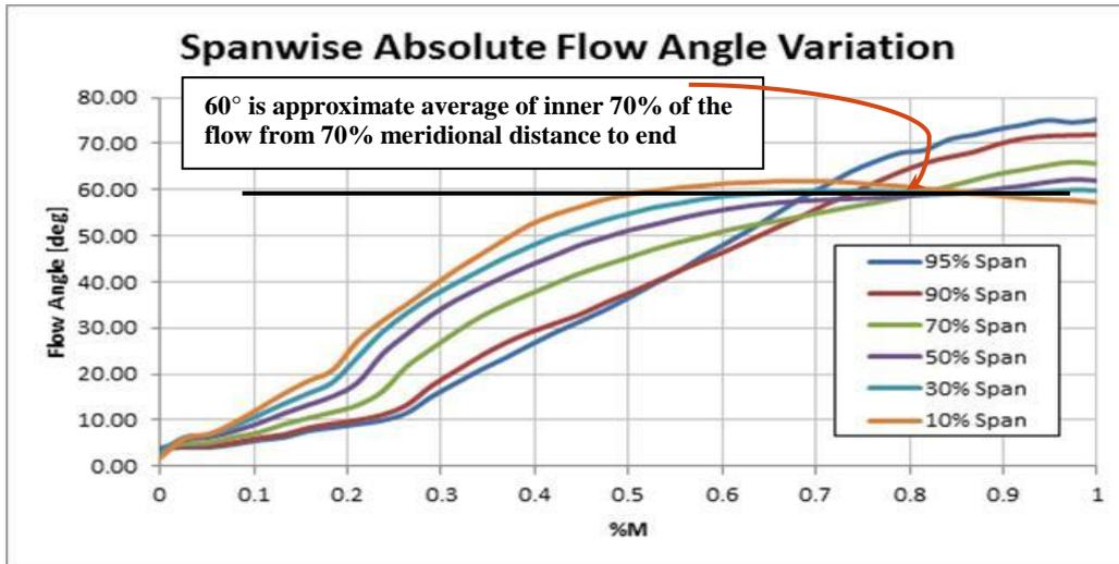
Figure 3. Blade-to-blade averaged flow angles at various % spanwise locations showing 1) crossovers at 70% - 80% meridional distance, 2) a group of angle traces that settle out to a level of about 60°, and 3) two traces that rise to higher angles; impeller at 4° incidence
