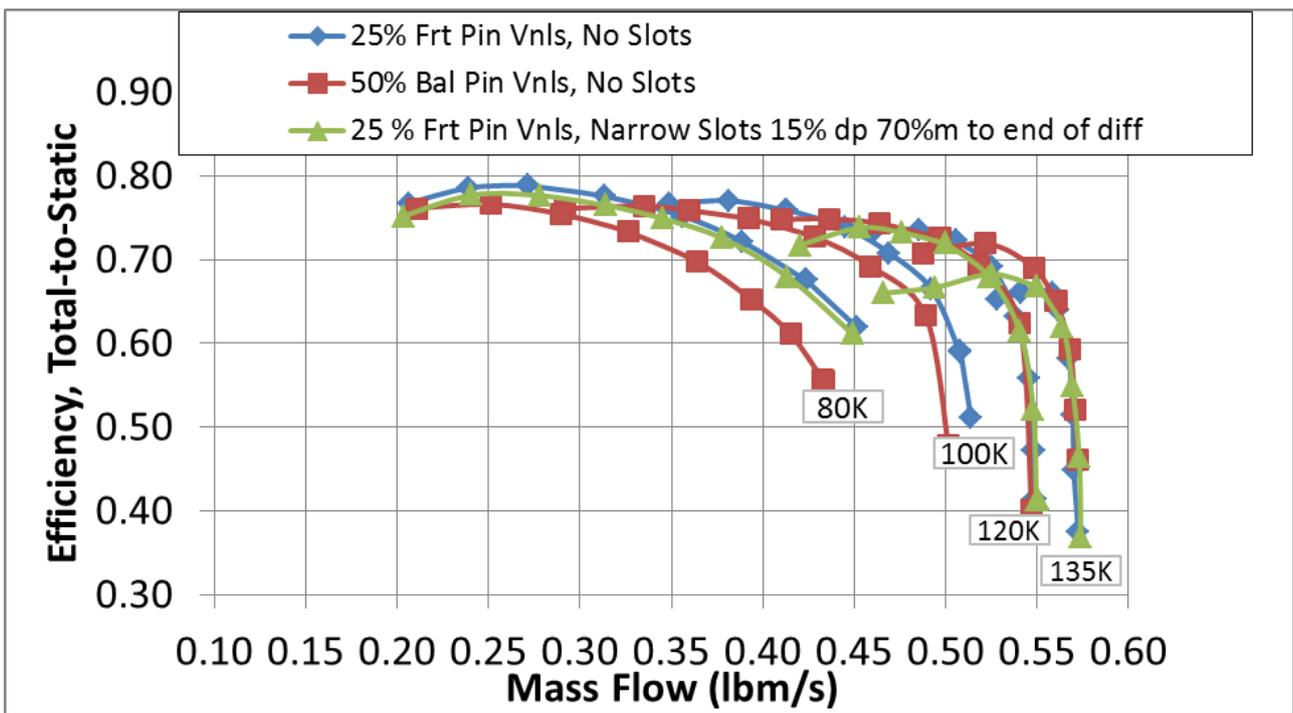
Figures 9a and 9b. Mixed diffuser pinch levels without grooves against the best grooves (to the diffuser exit); Figure 6b cover
