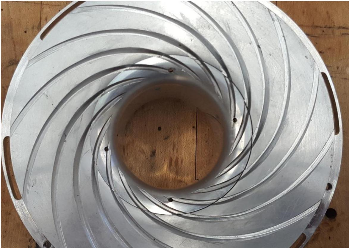
**Figure 6b.** The flow-wise grooved-cover (aka CCFG) showing the impeller cover below the reference circle and outside the circle is the diffuser front plate (25% front pinch configuration); grooves to end of the diffuser
