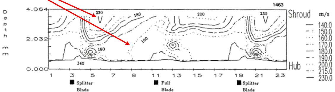
Figure 1b. L2F measurements:  $C_\theta$ ; near diffuser inlet,  $r = 1.1r_2$ ; 80 krpm, 0.303 lbm/sec
