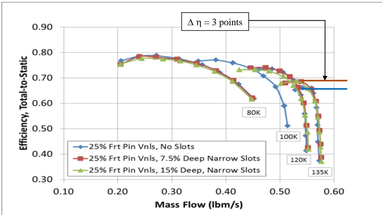
Figure 8b. Efficiency for the 7.5% and 15% deep grooves; Figure 6a cover
