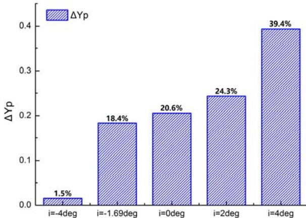
Figure 5. Relative Loss Coefficient over the Range of Operation
