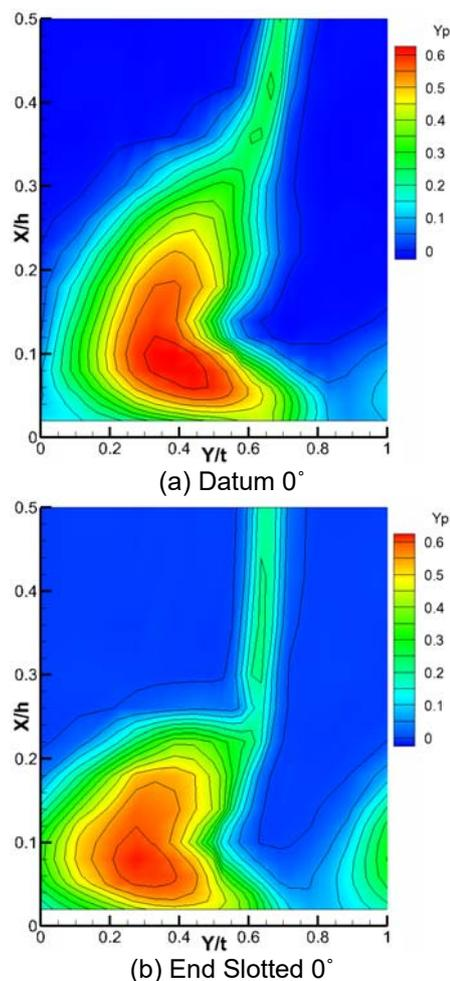
**Figure 8.** Measurement Plane Total Pressure Loss Contours under the incidence  $0^\circ$
