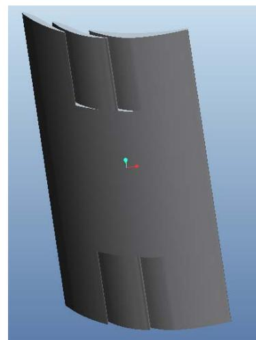
**Figure 1.** 3D Model of the End slotted blade
