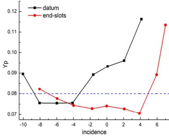
Figure 4. Total Pressure Loss over the Range of Operation
