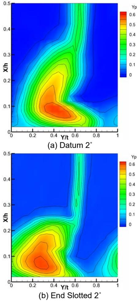
**Figure 9.** Measurement Plane Total Pressure Loss Contours under the incidence 2°
