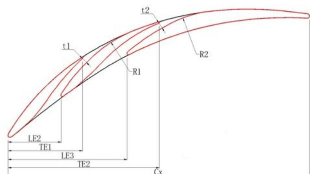
**Figure 2.** Cross Section Configurations of the Datum and End Slotted Blade Geometry
