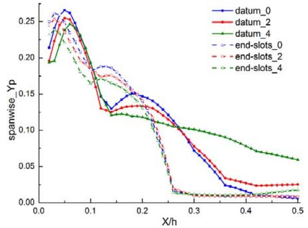
Figure 6. Spanwise Distribution of Pitch-Averaged Total Pressure Loss at the Measurement Plane
