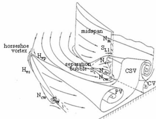
**Figure 11.** The Main Vortex Structures in the blade-endwall conjunction [21]
