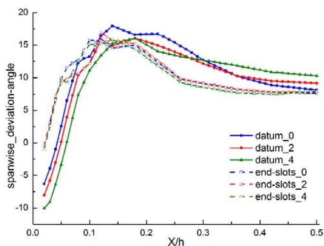
**Figure 7.** Spanwise Distribution of Pitch Averaged Deviation Angle at the Measurement Plane
