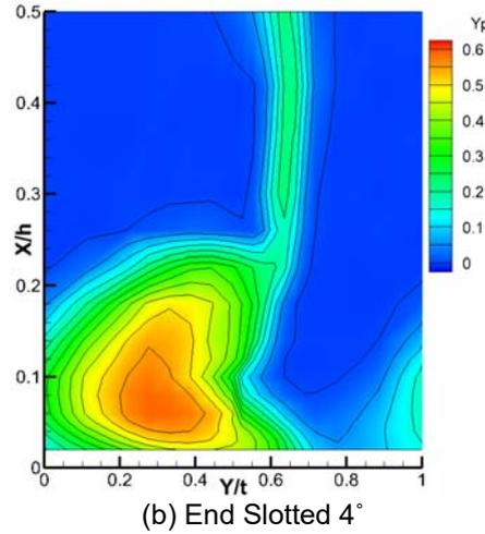
**Figure 10.** Measurement Plane Total Pressure Loss Contours under the incidence 4°
